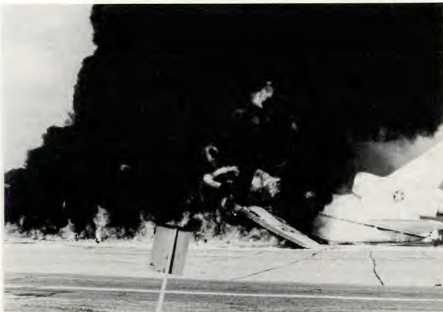
With JP-4's flashpoint below 0° F, there is always the potential for flammable mixtures in the aircraft fuel tanks. JP-4 leaking from a line coupling into a compartment containing electrical equipment and an arcing battery charger caused this disastrous KC-10 explosion.
