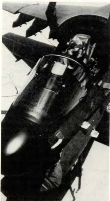
The new one-piece A-7 windscreen eliminates two large metal frame members. This allows the pilot unrestricted forward vision.
