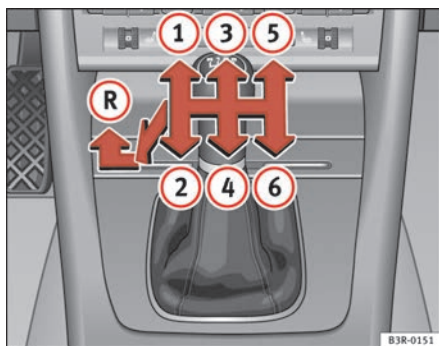
Fig. 145 Detail of the centre console: gear shift pattern of a 6-speed manual gearbox
