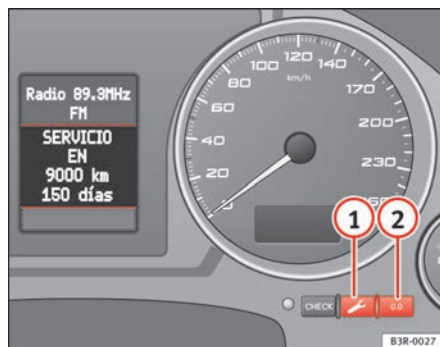
Fig. 51 Detailed view of the instrument panel: Service indicator
