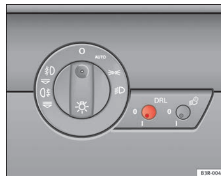
Fig. 88 Switch for daytime running lights
