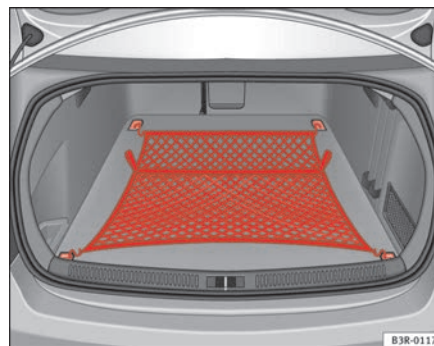
Fig. 116 Stretch net laid out
