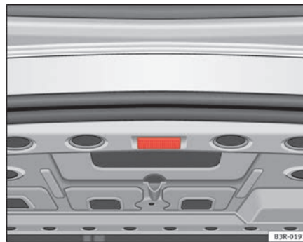
Fig. 95 Detailed view of the top of the luggage compartment: luggage compartment lighting
