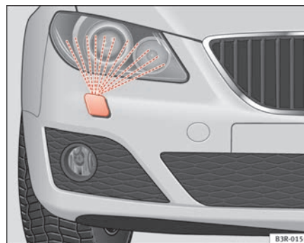
Fig. 101 Headlight with extended washer jet
