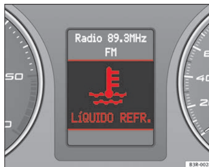
Fig. 53 Display: Coolant level warning
