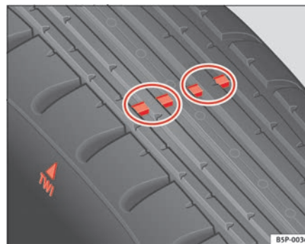
Fig. 173 Tyre tread wear indicators
