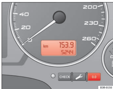
Fig. 42 Detailed view of the instrument panel: Distance display
