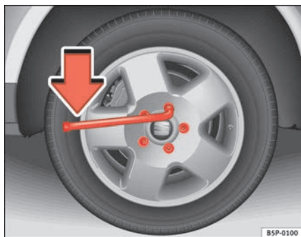
Fig. 178 Changing the wheel: Loosen the wheel bolts
