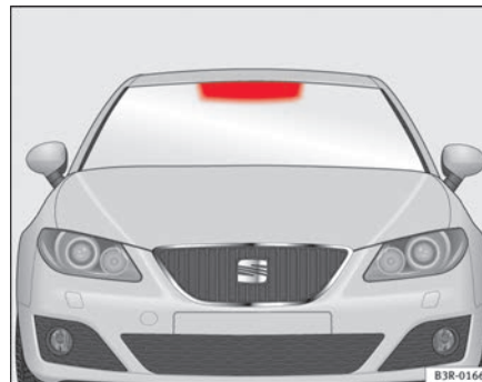
Fig. 159 Location of the electronic toll collection system
