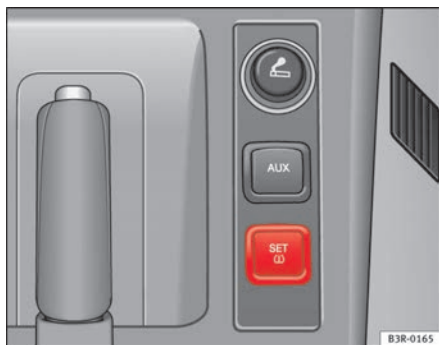
Fig. 172 Detailed view of the centre console: Button for the tyre pressure monitoring system
