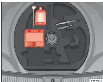
Fig. 176 Tyre Mobility System under floor panel in luggage compartment
