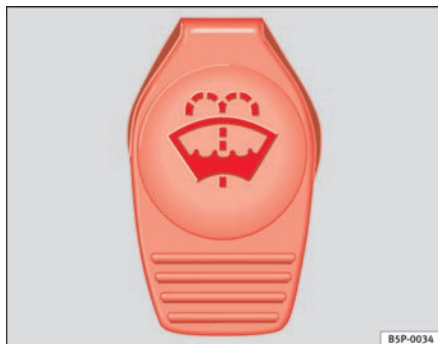
Fig. 168 In the engine compartment: Cap of windscreen washer fluid reservoir.
