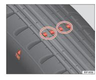
Fig. 134 Tyre tread wear indicators
