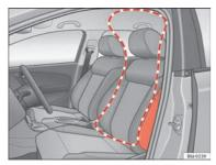
Fig. 20 Side airbag in driver seat
