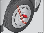
Fig. 136 Remove the complete hub cap
