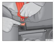
Fig. 15 Removing latch plate from buckle
