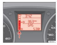
Fig. 31 Instrument panel: gas gauge.
