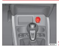
Fig. 87 Front power socket
