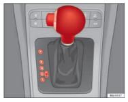
Fig. 108 Changing gear with tiptronic
