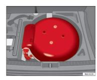
Fig. 121 LPG tank in spare wheel well
