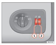
Fig. 56 Dash panel: regulation for instrument and switch illumination and headlight range control
