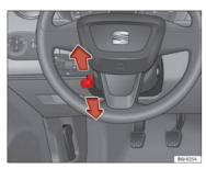
Fig. 97 Steering column height adjustment
