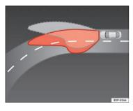
Fig. 57 Cornering lighting using adaptive headlights
