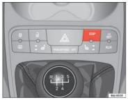
Fig. 98 Detailed view of the centre console: ESP button.
