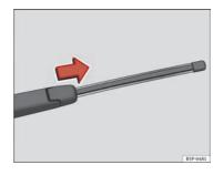
Fig. 131 Removing the rear window wiper blade
