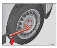
Fig. 137 Changing the wheel: loosen the wheel bolts
