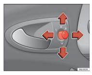
Fig. 68 Controls of exterior mirrors
