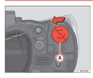
Fig. 144 Single turn signal lamp
