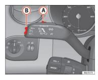
Fig. 112 Turn signal and main beam headlight lever: switch and rocker switch for the cruise con-
