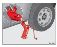
B6L-0047 Fig. 139 Fitting the jack
