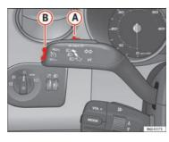
Fig. 114 Turn signal and main beam headlight lever: switch and rocker switch for the cruise control
