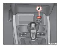
Fig. 100 Centre console: gas system control switch.
