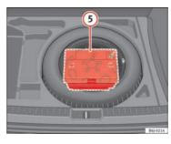
Fig. 174 For vehicles with the battery in the luggage compartment.
