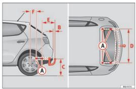
Fig. 118 Attachment points for towing bracket
