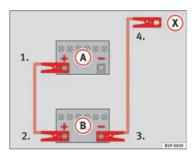
Fig. 168 Diagram for connecting jump leads if the vehicle providing assistance the current is not fitted with the Start-Stop system: flat battery (A) and battery providing current (B).
