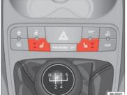
Fig. 73 Front seats heating switch
