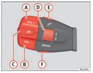
Fig. 42 Audio + Telephone Control
