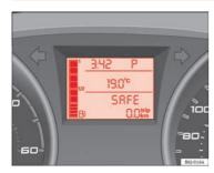
Fig. 36 Digital display: Gear lever position for automatic gearbox.
