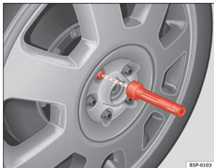
Fig. 154 Changing the wheel: Hexagonal socket in screwdriver handle to turn the wheel bolts
