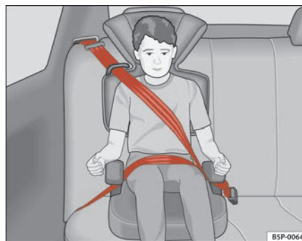
Fig. 29 Forward-facing child seat installed on rear seat.
