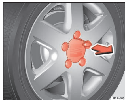
Fig. 150 Changing the wheel: Removing a hub cap
