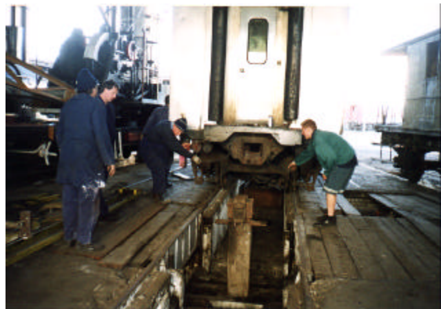
Robert Ralston, James Gray, Ben Parker and other members of Goulburn Roundhouse assist in the installation of the coupler and cushion block to the number one end of CF5010 on Saturday 20 July 2002 (John Horne)
