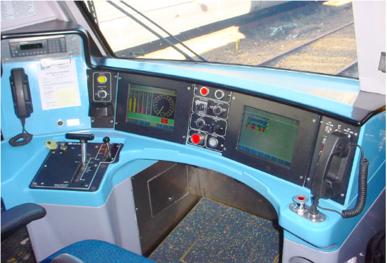
ABOVE: The driving controls in D1001 during the launch at Sydney Terminal. The desk-console layout of the controls shares some similarities with the Tangara's controls, but with a number of new features (John Clifton) BELOW: Set M2 picks up passengers at Rockdale on a Bondi Junction all-stations service on 8 August 2002. This station is currently undergoing a major upgrade (Paul Vonwiller)
