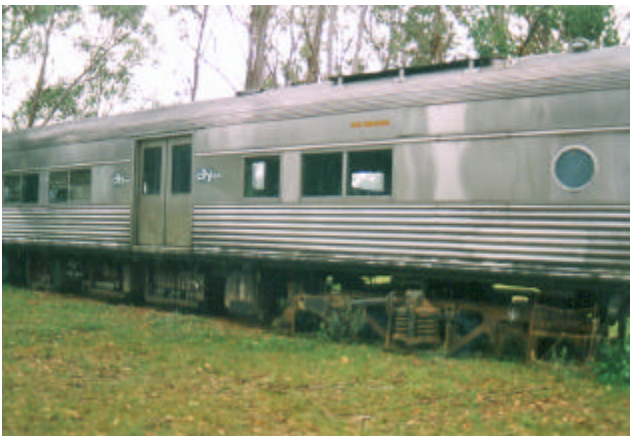
THE 'MATRIX' CAR. LEFT: During 1999, CF5025 was heavily altered into a facsimile of an American mass transit subway car for the movie "The Matrix". This car was recently re-used in the sequel of that same movie. A pair of sliding doors were cut into one side and an existing swing-door and window were plated over. While it's unfortunate that these alterations were done to one of the few CF motor-cars left in near-original condition, it must be admitted that these alterations have been expertly done! RIGHT: The alterations to the driver's end of 5025 and the unaltered off-side of the car. Compare this to the photo of the same car on page 93 (SETS Photos)
