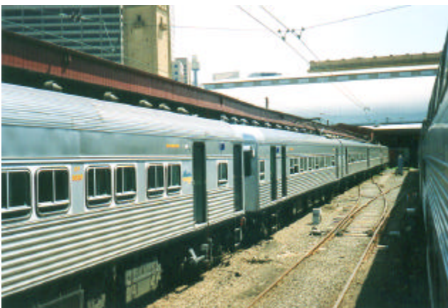
LEFT: The driver's end of CF5029 was extensively rebuilt after the 1973 fire at Gosford that destroyed cars CF5034 & ETB6033. Close inspection will see the separation marks on the letterboard and the roof. The original-window four-car set behind it had been used on a railfan tour a few days before this photo was taken in 1991 (Roy Howarth) RIGHT: One minor internal difference amongst the ETB trailers is the position of the roof vents in relation to the centre bulkhead. In this photo of ETB6028 taken from the former non-smoking compartment, one vent is directly above the bulkhead, hence the small opening for it at the top. Later ETB cars (possibly from 6030 onwards) don't have this feature as the vents are positioned on each side of this bulkhead The large windows on this bulkhead are non-standard features unique to the ETB cars (John Horne)
