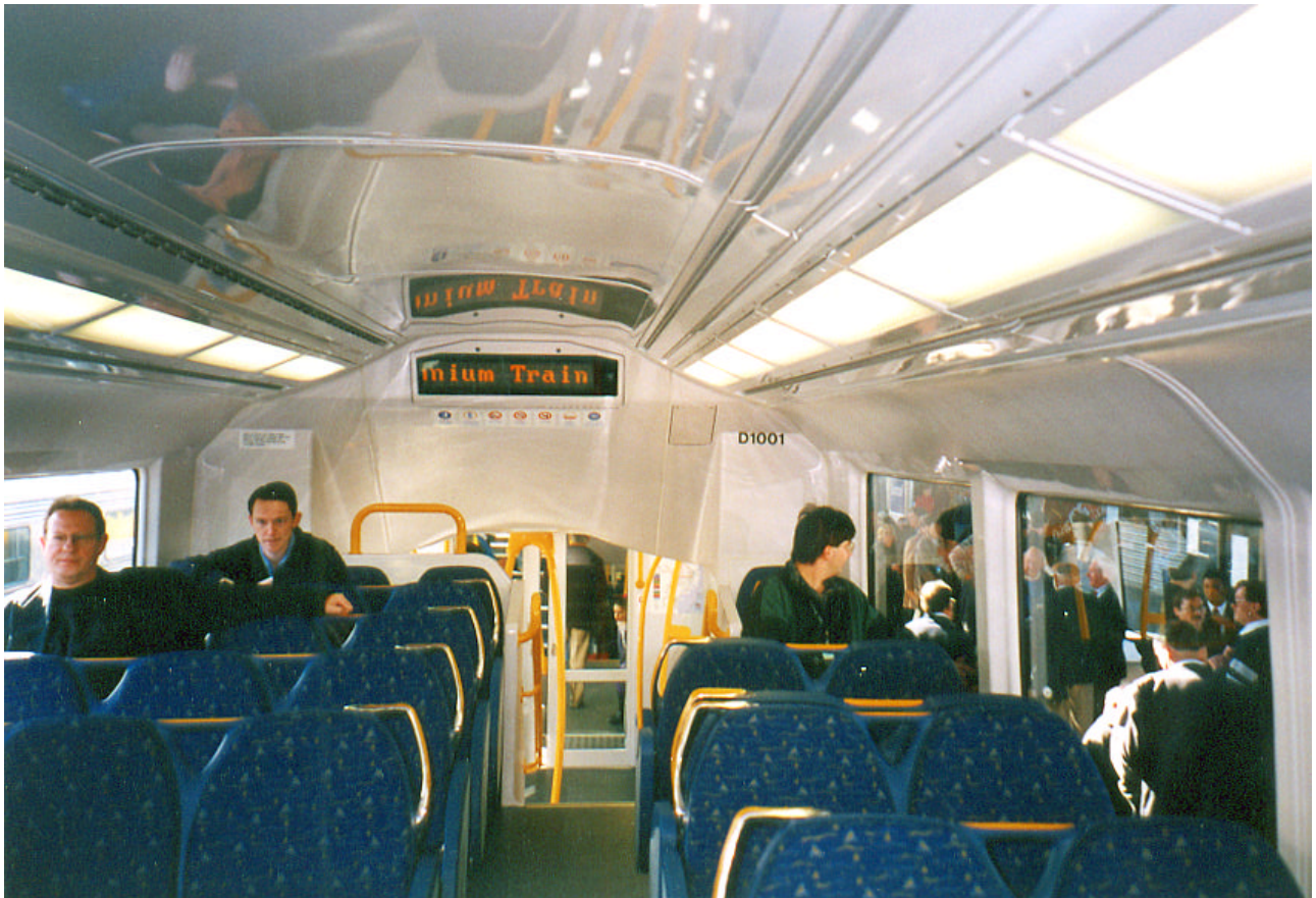
THE INTERIOR. ABOVE: The upper-deck of D1001 looking towards the No.1 (pantograph) end. Features to note are the electronic display (which has a security camera to the right of the display screen), the fabric seats with chrome seat handles and the roof contour (Paul Vonwiller) BELOW: The lower-deck of D1001 at Circular Quay on 5 July 2002. Unlike all previous double-deck cars, the lower-deck roof contour isn't flat, but slightly curved (Dominik Gientza)
