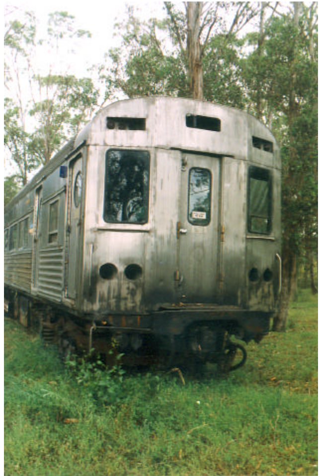
THE 'MATRIX' CAR. LEFT: During 1999, CF5025 was heavily altered into a facsimile of an American mass transit subway car for the movie "The Matrix". This car was recently re-used in the sequel of that same movie. A pair of sliding doors were cut into one side and an existing swing-door and window were plated over. While it's unfortunate that these alterations were done to one of the few CF motor-cars left in near-original condition, it must be admitted that these alterations have been expertly done! RIGHT: The alterations to the driver's end of 5025 and the unaltered off-side of the car. Compare this to the photo of the same car on page 93 (SETS Photos)
