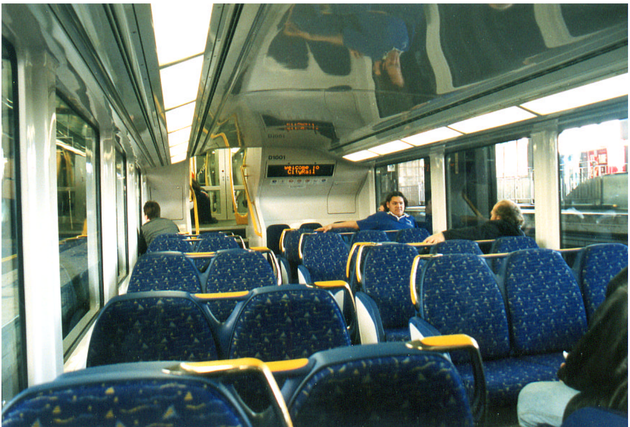
THE INTERIOR. ABOVE: The upper-deck of D1001 looking towards the No.1 (pantograph) end. Features to note are the electronic display (which has a security camera to the right of the display screen), the fabric seats with chrome seat handles and the roof contour (Paul Vonwiller) BELOW: The lower-deck of D1001 at Circular Quay on 5 July 2002. Unlike all previous double-deck cars, the lower-deck roof contour isn't flat, but slightly curved (Dominik Gientza)
