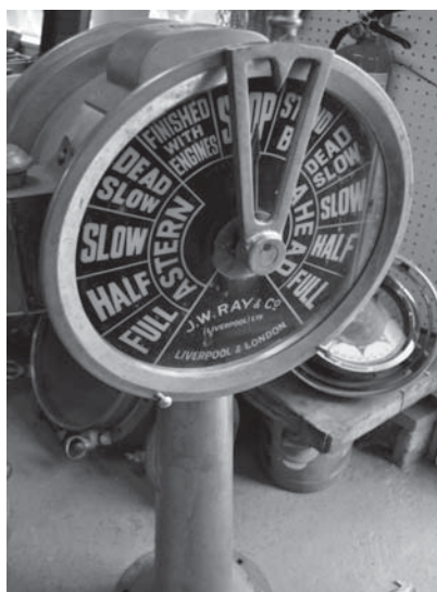
A ship's order telegraph, circa 1880, manufactured by J. W. Ray and Co. prior to the advent of ship's electricity. Photo courtesy Tony Kime, Annapolis Maritime Antiques
