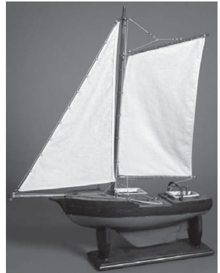
A fine handmade, circa 1895 pond model. The hull is made from one piece of wood roughly hollowed out. The mast, boom and gaff are original, as are all the deck fittings. Photo courtesy Dave White, White's Nautical Antiques
