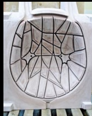
Mold made by Vitra for producing models in vacuum-cast resin, 2008
