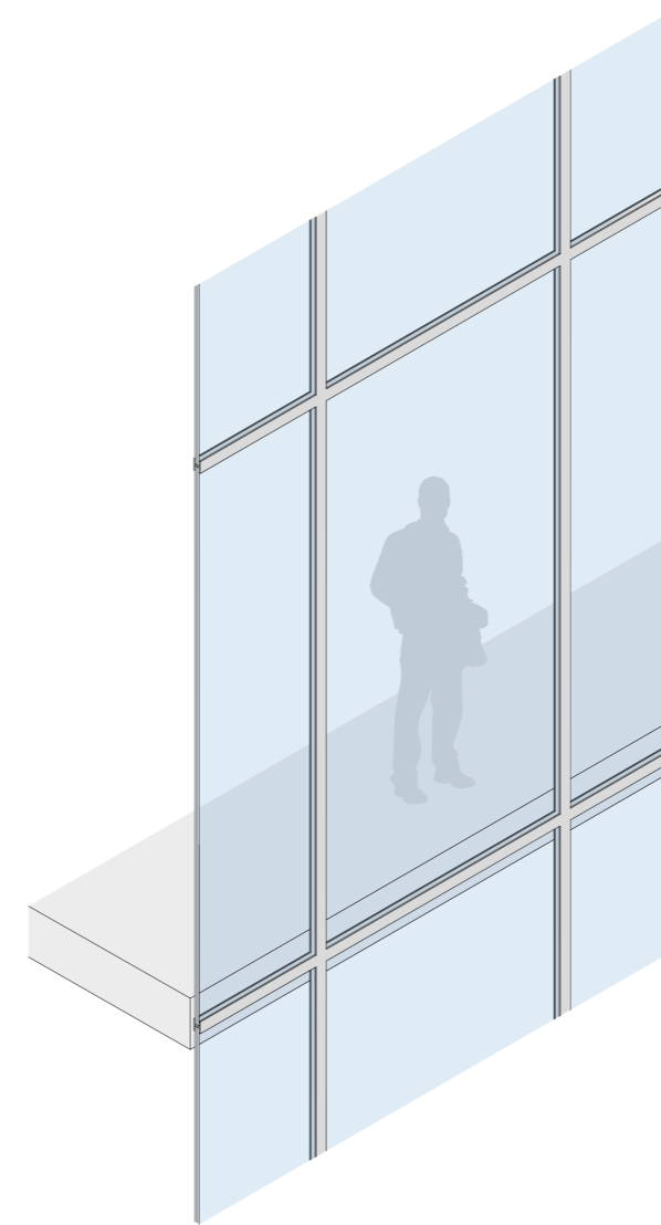
Conventional, 4-sided linear support in a framing system that uses gaskets ('dry-glazing') or bonded with a structural sealant ('wet-glazing').
