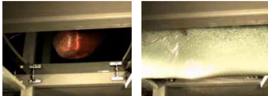
canopy test / SentryGlas® 0.89 mm (35 mil) / 100 kg (220 lb)
