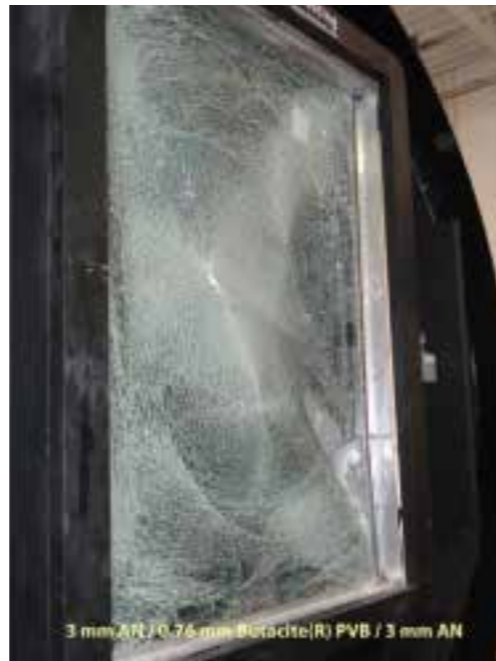
A post-blast test image of one ionoplast laminate is shown in the picture on the right and an image of a PVB laminate is shown in the picture on the far right.
