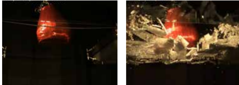
canopy test / tempered glass / 50 kg (110 lb)
