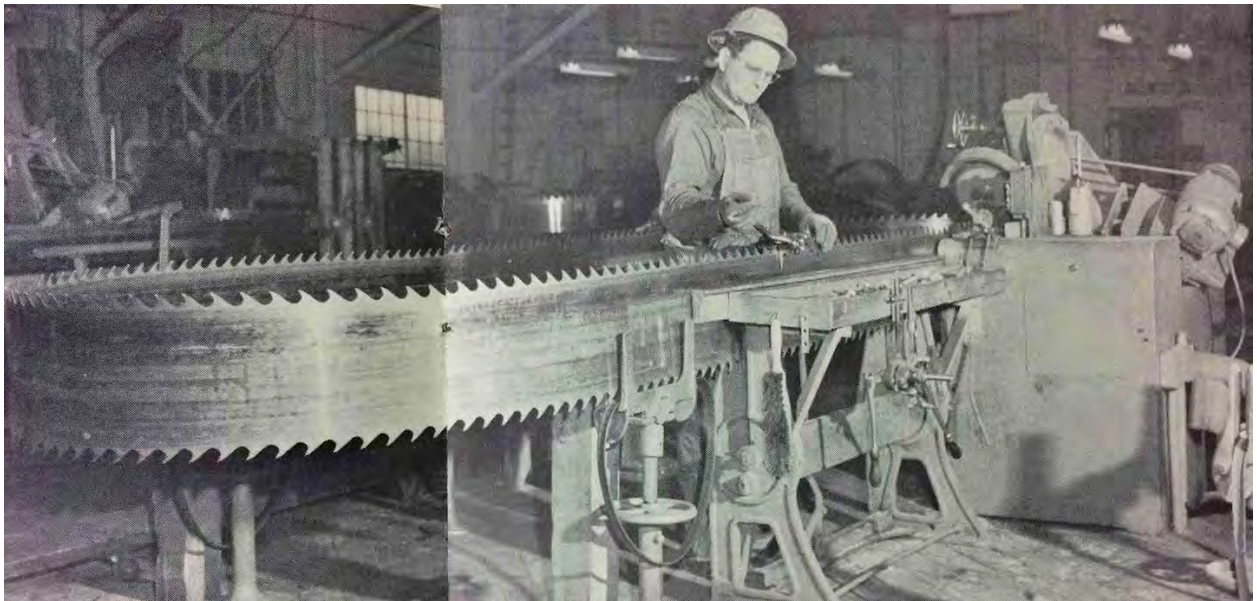
Figure 29. Modern band saw being repaired at Weyerhaeuser mill, circa 1954. From "Welcome to Springfield Branch Operation" by Weyerhaeuser Timber Company.
