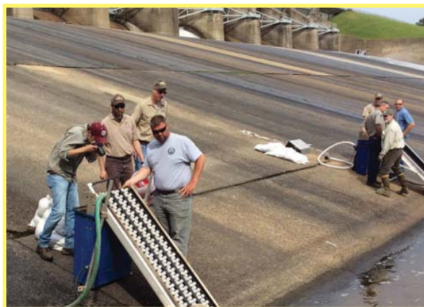
WRB staff and state and federal agencies evaluate eel passage ramp setup.
