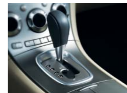
5-speed Electronic Direct Control Automatic Transmission with SPORTSHIFT® (SEAT SS)
