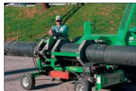
McElroy T630 Fusion Machine 8" IPS – 24" pipe
