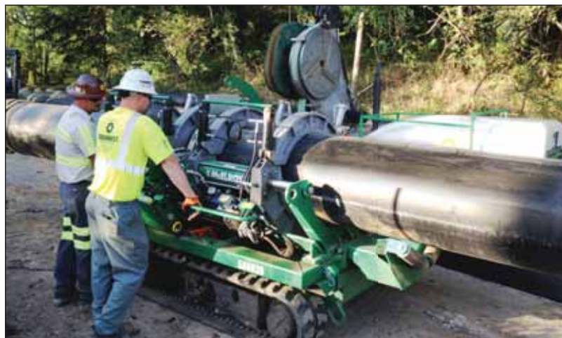
McElroy T630 Fusion Machine 8" IPS – 24" pipe
