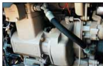
Direct-Drive Air Compressor Eliminates maintenance problems common to belt-driven compressors
