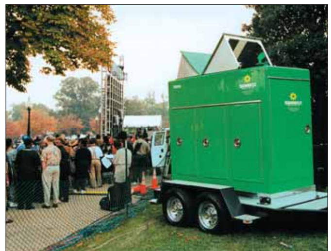
Crawford 1,400 amp Movie Set Generator Powering video screens at an outdoor rally
