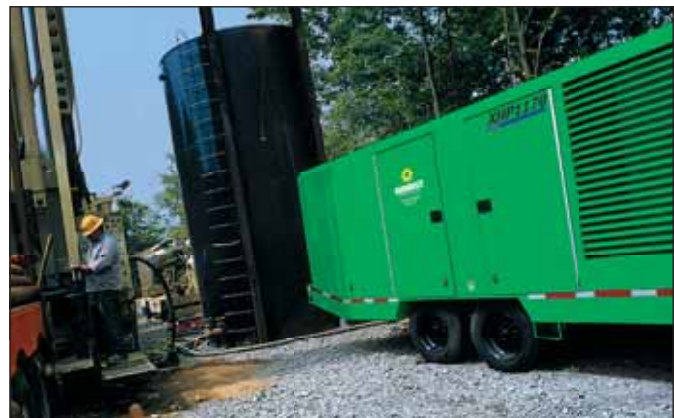
Doosan XHP1170 1,070 CFM High-pressure Air Compressor, 350 PSI
