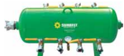
Tank-Type Air Manifold (8) ball valve controlled outlets 2" air inlet with 4-prong coupler on one end and flow-through plug on other end allows using multiple units in tandem. Texas Pneumatic TX-2AMF
