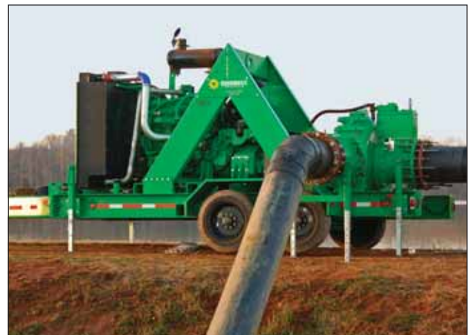
Premier 24" x 24" Diesel Trash Pump Working on an emergency dewatering project
