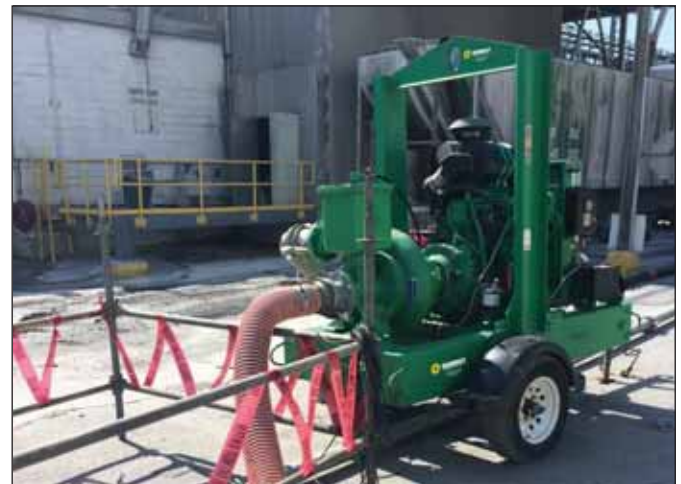
Gorman-Rupp 6" x 4" Diesel Trash Pump Working on a construction dewatering project
