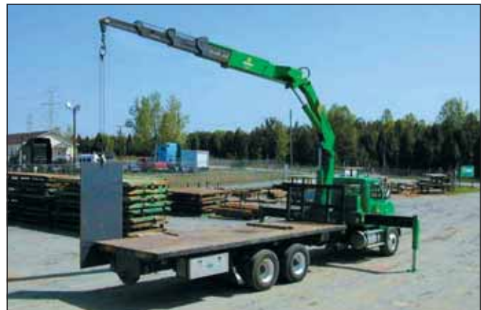
Pump & Power locations are equipped with boom trucks that can deliver road plates and other trench shoring equipment
