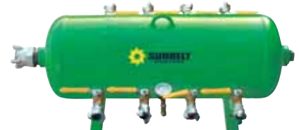
Tank-Type Air Manifold (8) ball valve controlled outlets 2" air inlet with 4-prong coupler on one end and flow-through plug on the other end allows using multiple units in tandem. Texas Pneumatic TX-2AMF
