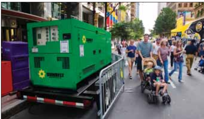
MQ Power 100 kW Towable Generator Temporary power for food vendors during a street fair
