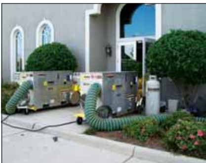
2,000 CFM Gas Desiccant Dehumidifiers
