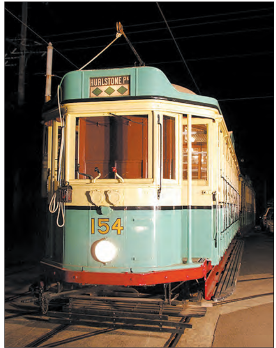
L/P car 154 stands under the floodlights on 24 June. It is carrying a traditional kerosene tail lamp. If the trolley pole dewired and the tram was plunged into darkness, the kerosene lamp would provide some warning to oncoming traffic in the days when road traffic was much lighter than it is today.
