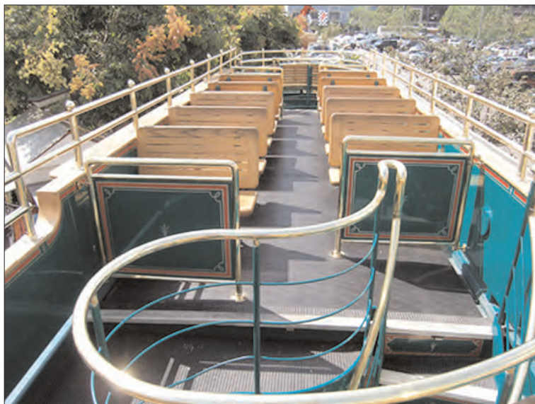
The top deck has 2 x 2 fixed seating with additional seats around the staircases at the ends of the car. John Smatlak
