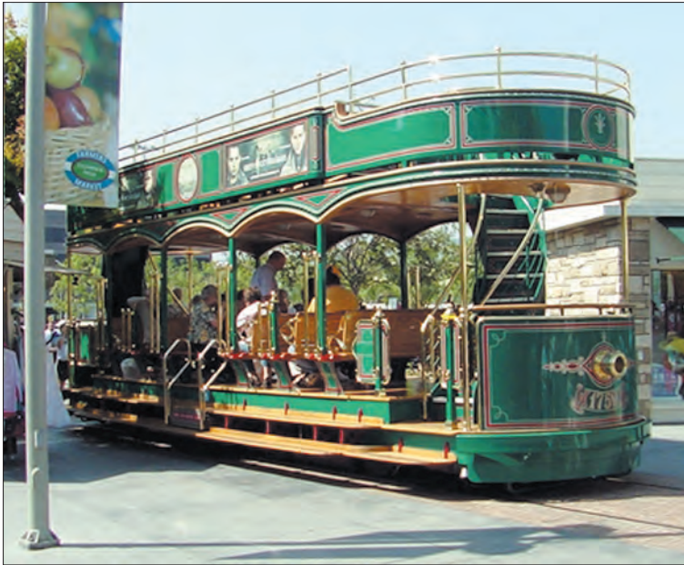
This view of the trolley shows the position of the cassette wheelchair lift which doubles as a stairway. John Smatlak
