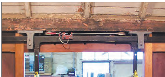
The Sydney J car door mechanism which allows the operation of one of the pair of doors to also open the opposite one. Bendigo Tramways
