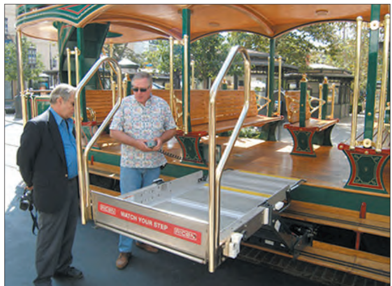
A cassette type wheelchair lift which fits under the floor and wheelchair tie down points are provided.
