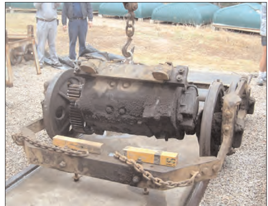
On 20 June, the motor from one of Dreadnought 136's Brill 39E trucks was lifted out for overhaul.
