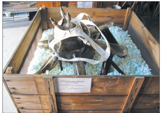
A new arrival from Melbourne is this mercury arc rectifier bulb still in its packing case and showing the special sling. Peter Hyde
