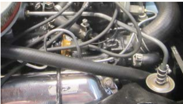
FOMOCO 2 bbl, Part No. C4DF with metal fuel line
