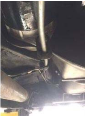
Clamp and routing of line past bell housing. Note: Rubber section of line around bell housing is CORRECT.
