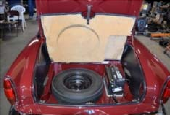
Mk1/Mk1a: Spare tire bolted down
