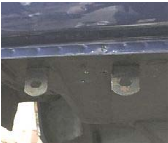
Formed twisted steel hangers affixed to brackets welded to underside of body
