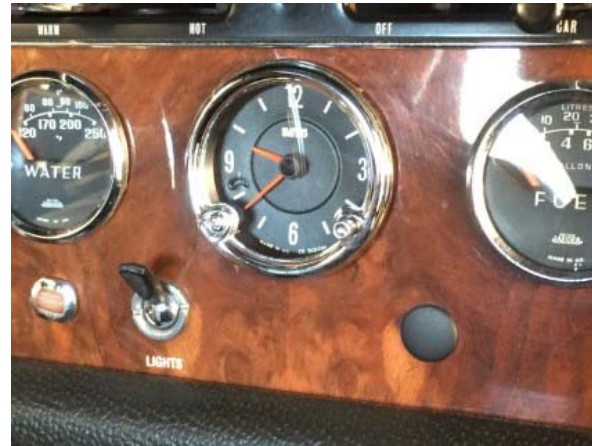
Wood Dash: Overdrive and cigar lighter hole chrome. Choke hole black wrinkle
