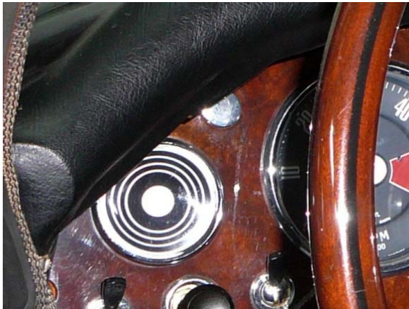
Wood Dash: Overdrive and cigar lighter hole chrome. Choke hole black wrinkle
