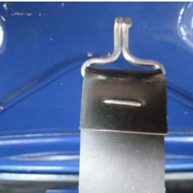
Mk2: Black rubber one inch strap with three piece bail wire hook that latches directly to underside of trunk lid. No footman loop or holes for the footman loop.
