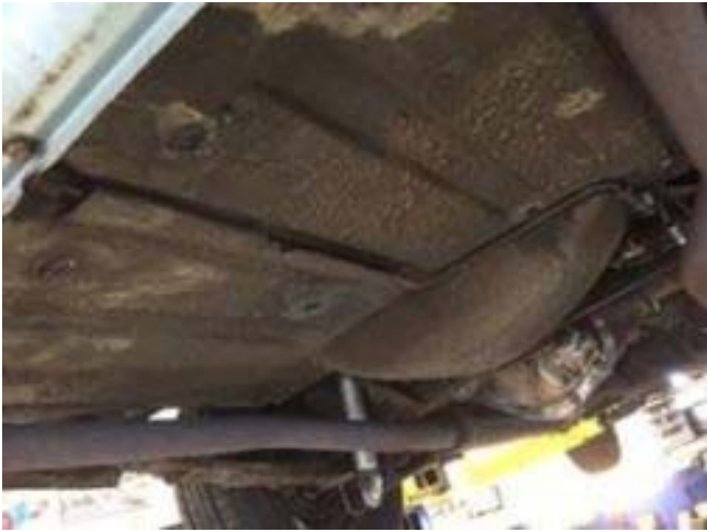
5/16" Steel, OEM Routing from fuel crossover to fuel pump
