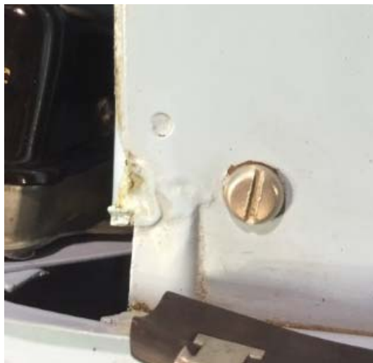
Unfinished slotted screw front/ left of scuttle panel
