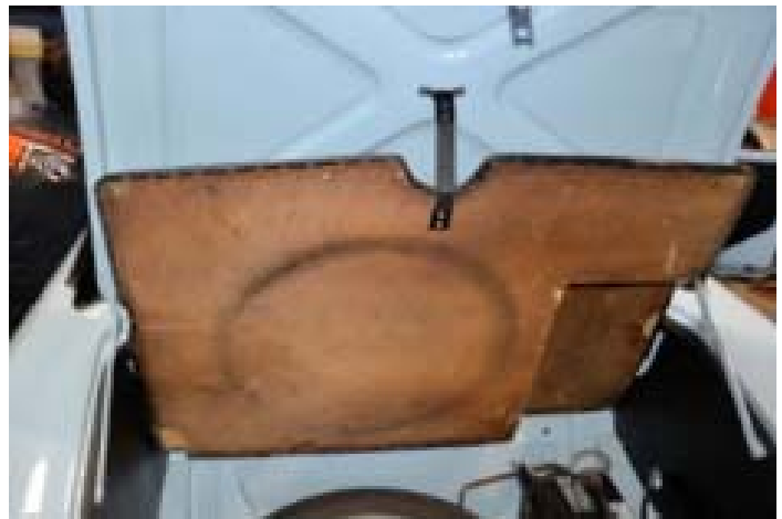
Mk1/Mk1a: Secured open with black vinyl strap with hook formed from sheet metal. Strap hooks to footman loop affixed to underside of deck lid
