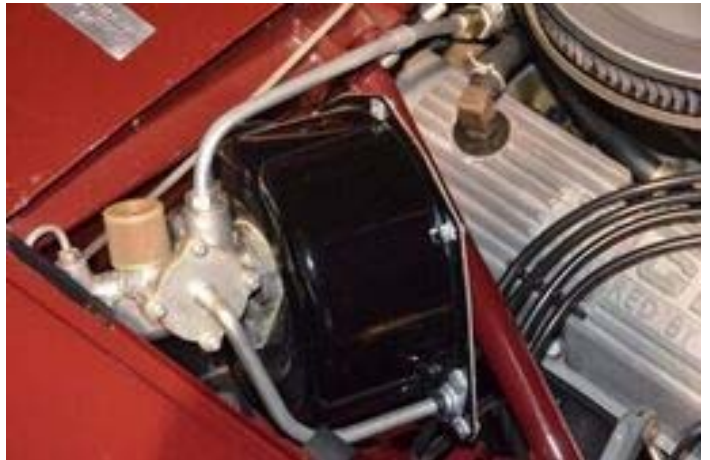
Late Mk1a/Mk2-Seven inch booster with hard vacuum line (exact point of production change unknown at this time.)
