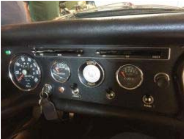
Mk1: (up to 9470400 est.) Black Vinyl dash Mk1: Heater Demister Controls: Metal with Chrome knobs Lower Dash pad material: Long Grain
