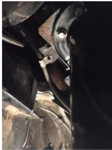
Clamp and routing of line as it turns upward at front of engine
