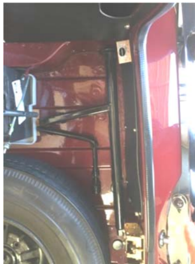
Mk1a/Mk2: Longer jack with base outboard and lug wrench inboard
