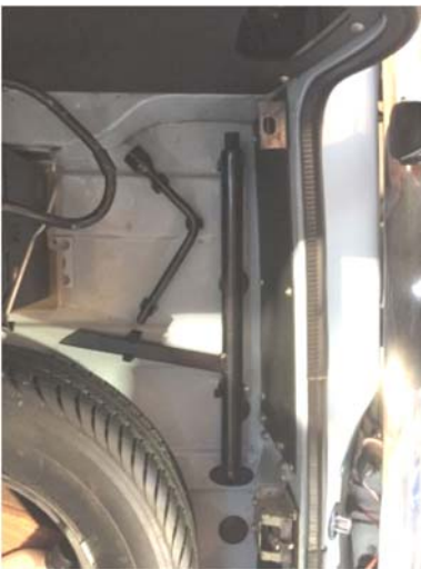
MK1 Short jack with base toward center and lug wrench outboard
