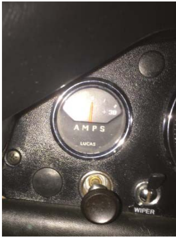
Black Vinyl Dash: All Black, Wrinkle Finish. Some have chrome plug in choke hole
