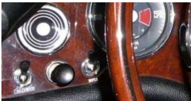
Mk1a/Mk2: Lower dash pad material: Pebble Blower Switch
