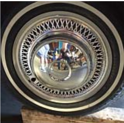
Wheel Trim Rings with Caps: Criss-Cross Style Mk1, up to 9473168
