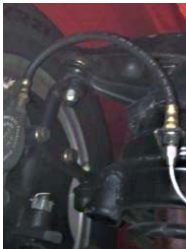
Brake Line: Hose secured by OEM fitting and clip (Clip missing: see close-up at right)
