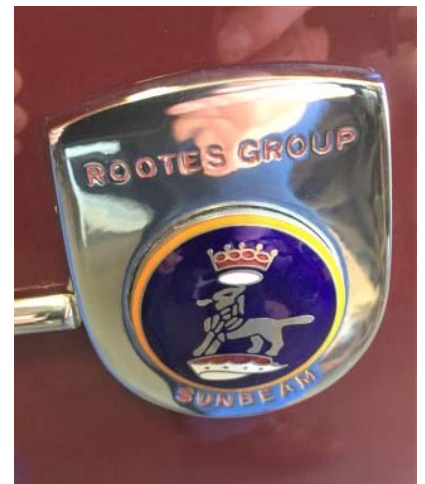
Reproduction rear quarter badge: Raised center disc. Lettering less defined
