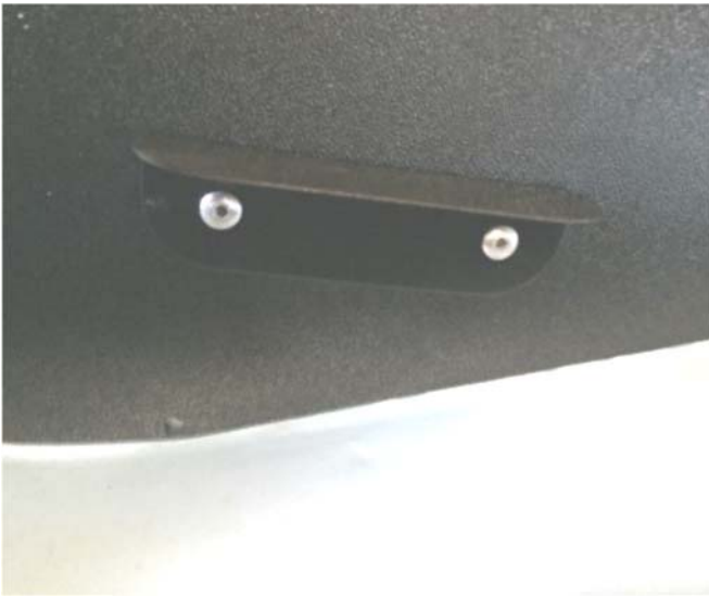
Mk1: Small bracket driver's side, large bracket passenger side.
