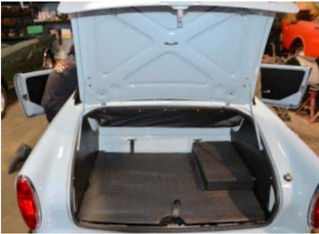
Plywood vinyl covered.
