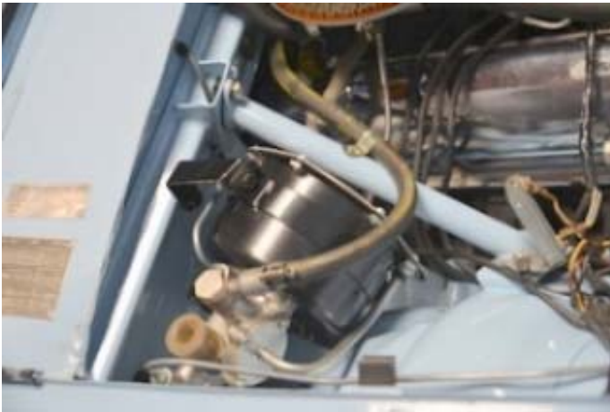
Mk1 and early Mk1a-Five inch booster with yellow striped rubber vacuum hose
