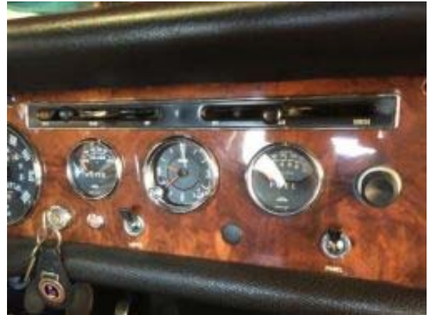
Wooden Dash for remainder of production Mk1a/Mk2: Heater Demister Controls: Metal with black knobs
