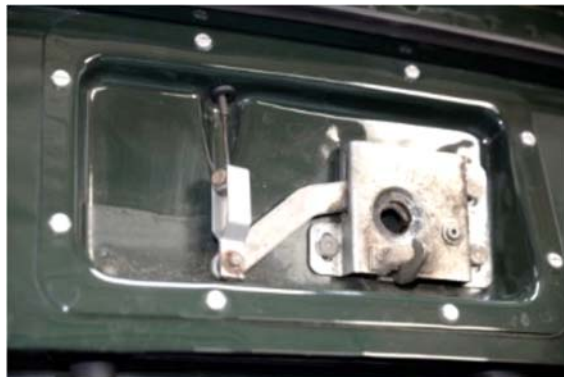
Mk1a/Mk2 Cable release
