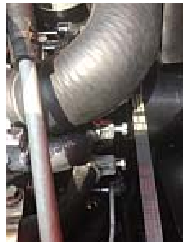
Ford Screw-type (tower) clamps.
