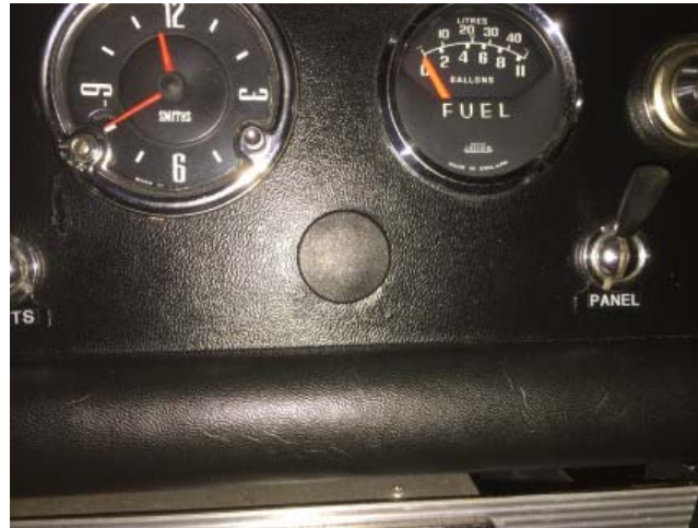
Black Vinyl Dash: All Black, Wrinkle Finish. Some have chrome plug in choke hole
