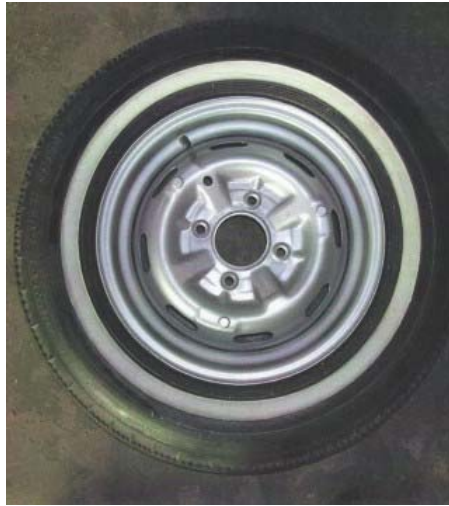
Later factory steel wheel (reinforced) Mk1a/Mk2
