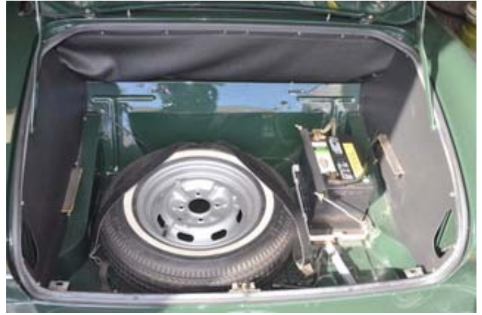
Mk2: Spare tire secured by straps/fuel pump in wheel well.
