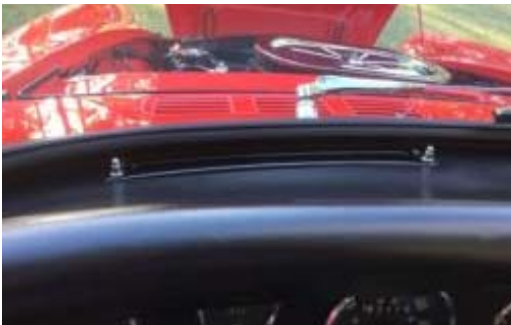
Early Mk1: Screwed into demister vent holes
