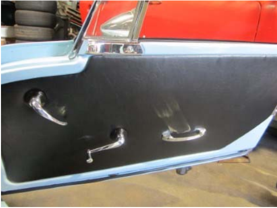
Mk1: Body color around perimeter, window crank located lower on panel
