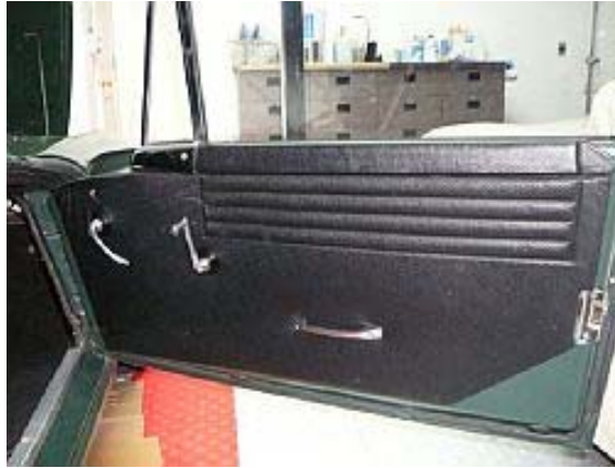
Mk1a/Mk2: Panel up to window, rolled material at top, window crank higher
