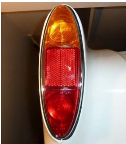
Amber turn signal lens, inside screw only for non-U.S. market
