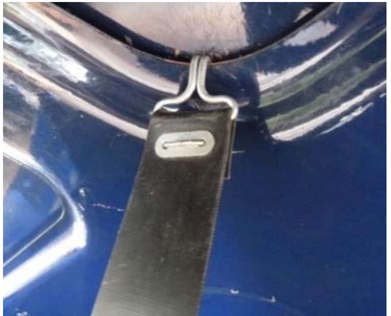
Mk2: Black rubber one inch strap with three piece bail wire hook that latches directly to underside of trunk lid. No footman loop or holes for the footman loop.
