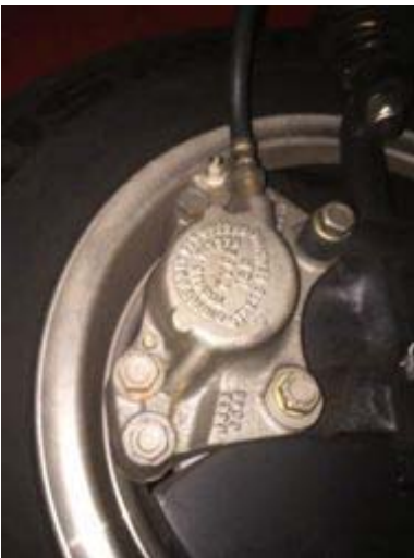
Calipers: bare steel finish
