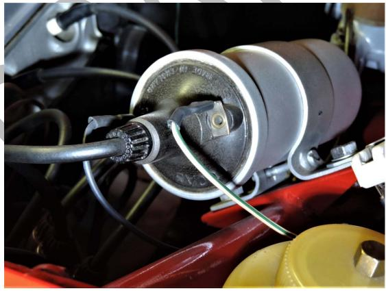
Series IV from B9410268 through end of production: Same as Series 3-IV but coil now has "Push In" connector on main terminal.
