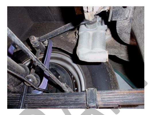
Series 3-V: The shock absorbers were changed to telescopic dampener type shock absorbers and the rebound strap was eliminated.
