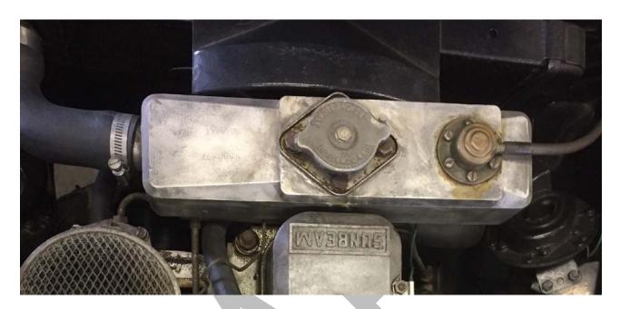
Series 3 through V: Radiator and fan shroud painted black. Fill cap now on radiato. Upper radiator hose runs directly to water neck on intake, No expansion tank.
