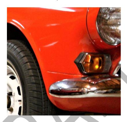
Series I-IV: Cars with round doors, hood and trunk have leaded body seam below front edge of door but no seam below rear corner.
