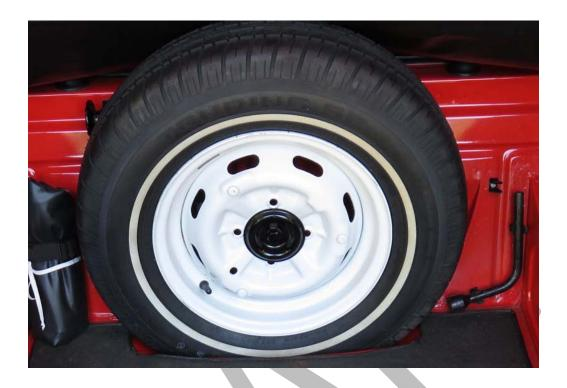
Series V: Spare is positioned vertically in well along front bulkhead and is secured with two straps.
