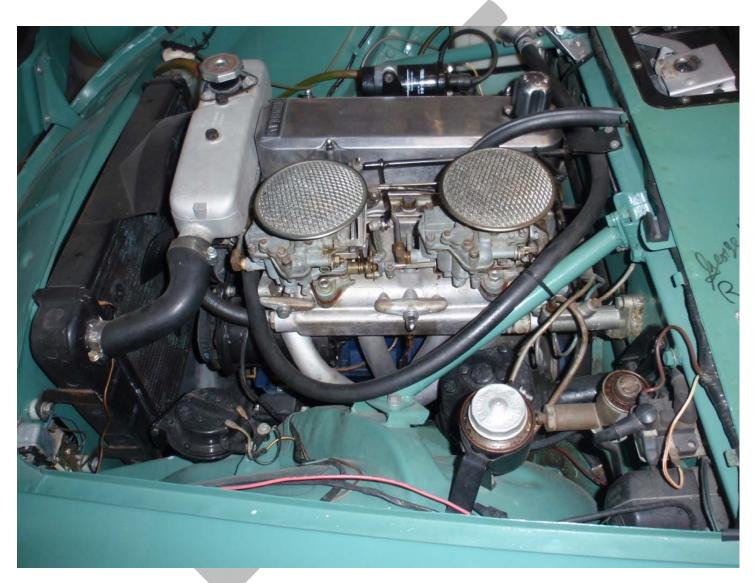
Series II-3: 1592 cc with twin Zenith carburetors. (Note: hose clamps and some wiring not correct.)
