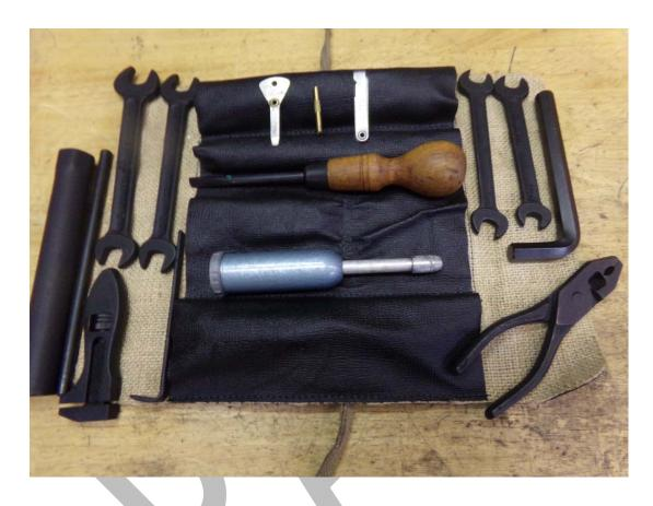
Series IV-V: Tool's are wrapped in a black all vinyl tool roll that is tied closed with an off white cloth tie strap. It is affixed by a black canvas strap to the front bulkhead left of the spare tire.
