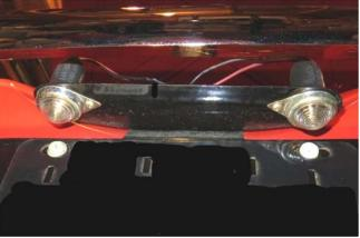
Series V from B395016692 (Between 16692 and 16779 some cars were produced with the older version license lights): Affixed to top of bumper with chrome covers backing the lenses.
