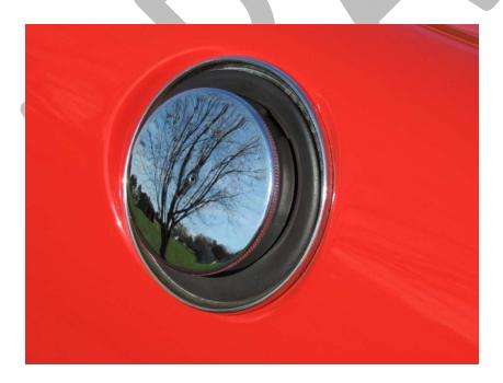
Series IV-V: Oval chrome cap with push button locking mechanism. Push button toward rear.
