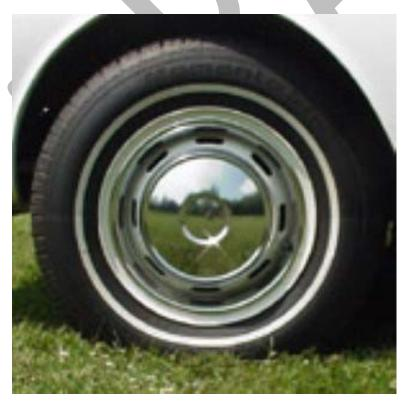
Series IV (B94102174 onwards): 8 hole steel wheel painted foam grey. New spoked trim ring design not equipped on spare.
