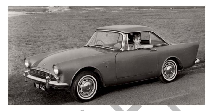
Series IV: Fins were greatly reduced in size. Rear is more squared off with redesigned tail lights, Round corners on trunk, hood and rear corner of door.
