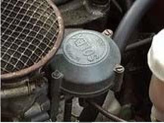
Series V: Twin Stromberg 150 CD carburetors. Carburetors are marked on top 150 CD STROMBERG The Zenith CARBURETTORS
