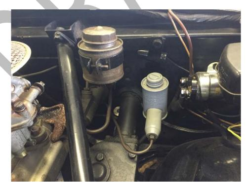
Series IV and V: Both clutch and brake master fluid reservoirs are affixed the firewall. The brake reservoir is just inside the left reinforcement bar and sits high along the forward edge of the scuttle. The clutch reservoir is positioned lower, just outboard from the left reinforcement bar. Both reservoirs have plastic caps.
