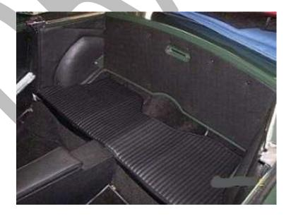
GT: No soft top compartment adds extra room. Side and back panels have padded black waist roll on top with four pleat rolls same as door panels. Padded seat cushion and sides are the same material and color as seats and door panels
