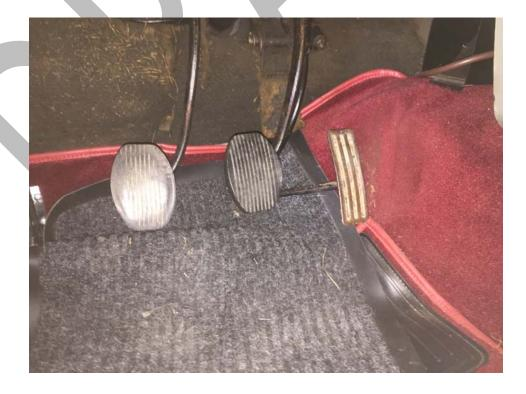
Series 3-V (up to B95002286): Accelerator pedal is organ type with base affixed to floor and rubber coated. Brake and clutch pedals same as Series II.
