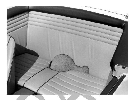
Series V: Tonneau cover to secure folded down rear top introduced. Covering on back and rear panels is incorporated as part of the tonneau cover. Back panel has a cushioned more rounded waist roll and five pleat rolls. Side panels are completely covered in vinyl and are the same color as seats. Full carpeting.
