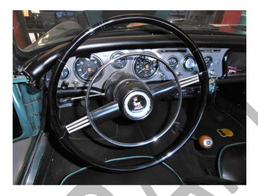
Series 3 to end of production ST: Black plastic with black plastic center cap with crinkle finish; three parallel spokes each side from center. Horn ring with two black spokes from center each with two oval holes.
