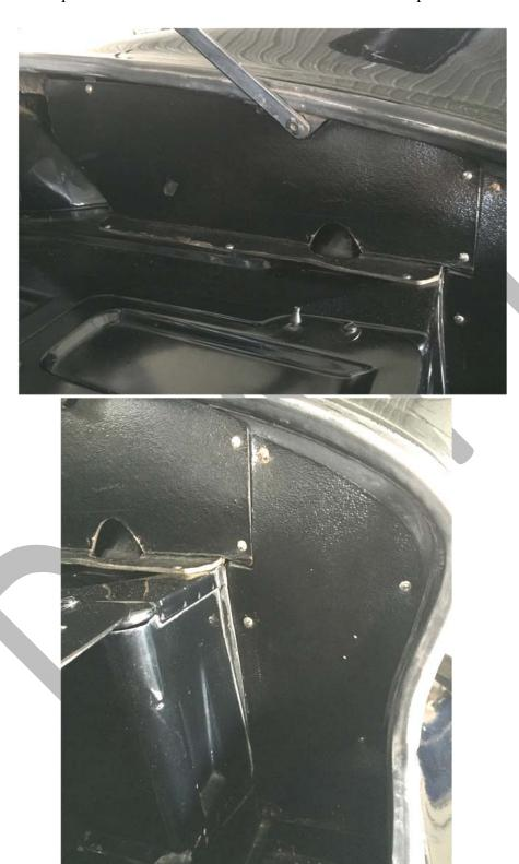
Series 3-V: One piece fiberboard panel with black wrinkle finish, affixed with Phillips head machine screws and cup washers.
