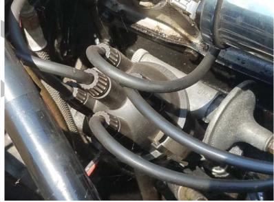
Series IV from B94202678 through Series V: Black cap more domed at top with longer, push-in type terminals. Located at right rear of engine block. (*Note: Green plug wires not correct.*)
