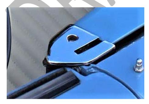
Series IV-V: Series 3-early Series V cap has fatter profile; Series V from 395004201 ST and 395004266 GT narrower profile cap
