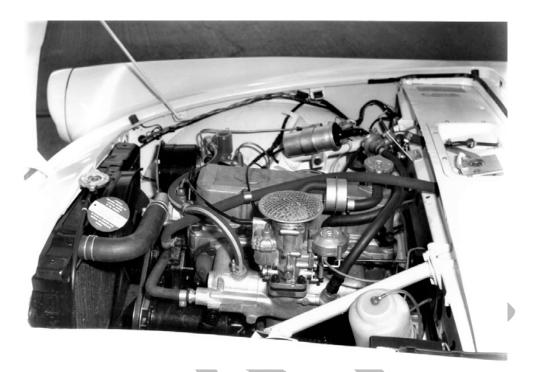
Series V: 1725cc with twin Stromberg carburetors (Note: orange spark plug wires not correct)
