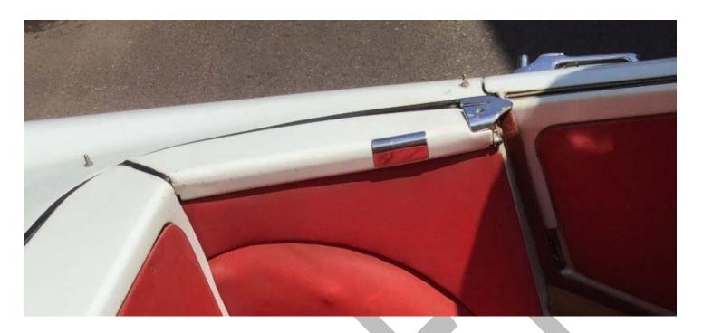
Series 3 and IV ST: The vinyl soft trim pad on the back panel is the same material and color as the seats and is affixed with twelve visible plastic rivets matching the color of the pad. The pull handle for the control cable is now recessed into the panel. The chrome piece on the side panel cover runs the full length of the inner edge,
