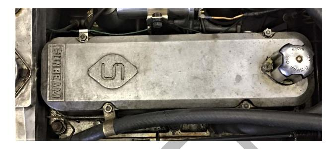
Series II and 3: From B9118448 to B9204717 ST and B9203886 GT: Same as Series I and II but filler neck at rear now has a tube opening on left for breather hose and a more traditional cap with USE SHELL OIL ONLY markings. Need Photo
