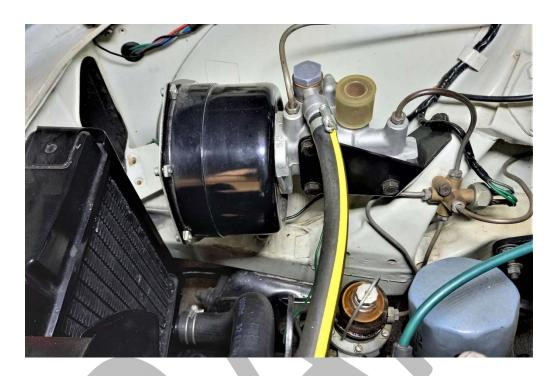
Series IV from B9402899 ST and B39402921 GT to end of production: 7" Servo
