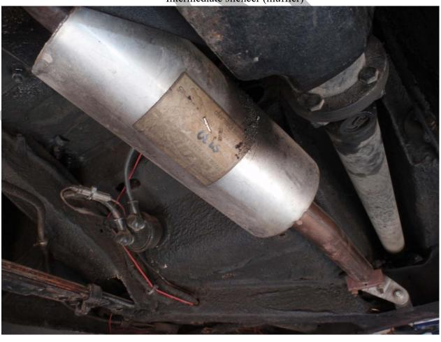
Primary silencer (muffler) and tailpipe (Note: Chrome tail pipe not correct.)
