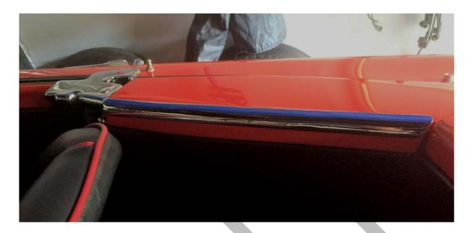
GT: No soft top compartment. Back and side panels are fully upholstered to match seats and have cushioned waist roll and four pleat rolls at top. Waist roll is black regardless of interior color.
