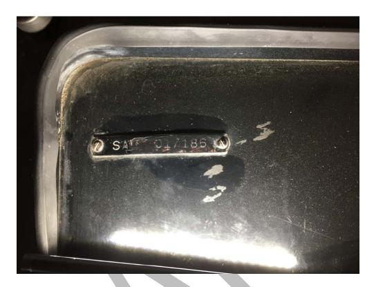
Series 3-IV: Steel VIN tag for Series 3, aluminum for Series IV, SAL tag painted body color and a recommended fluids tag all on the right side of scuttle panel. VIN tag includes ID number and paint code.
