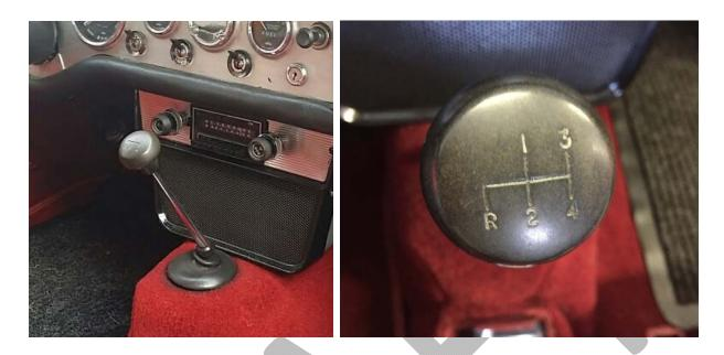
Series IV after B9405885: Gear shift lever knob changed upon introduction of fully synchronized transmission. Same shape, but reverse to the right and down.
