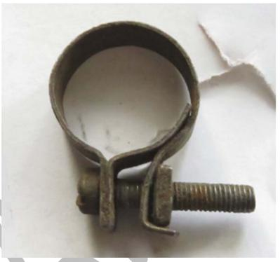
Sardine Clamp used on brake servo vacuum hose at servo end.
