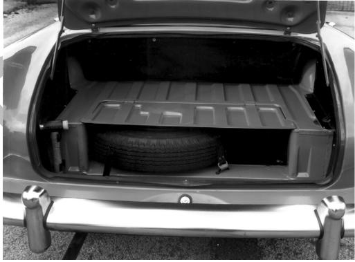
Series 3-V: Trunk compartment and underside of lid painted body color. Spare repositioned vertically at front of trunk area. Black rubber floor mat. Left photo Tool bag secured by strap left of spare secured by bolt; crank handle (*missing*) and lug wrench to right of spare. Right photo shows wire wheel equipped Series V cars with knockoff hammer and spare secured by straps. Bottom photo is from Rootes Sales Brochure showing layout for wire wheel equipped car.
