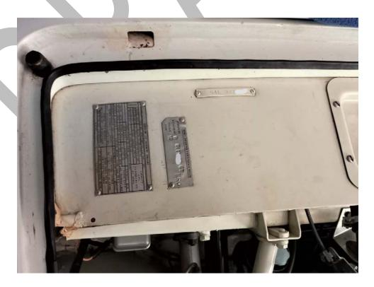
Series V: VIN tag (aluminum) affixed with rivets and SAL tag affixed with slotted screws and painted body color at right corner of scuttle panel. Recommended fluid tag is dropped.
