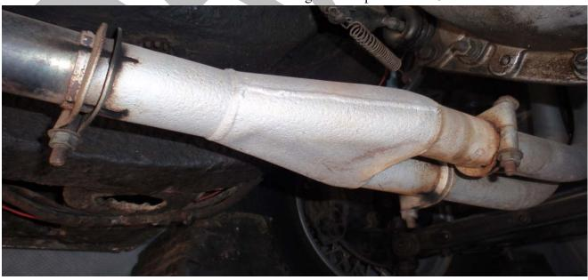
Y connector with original clamps on Series 3
