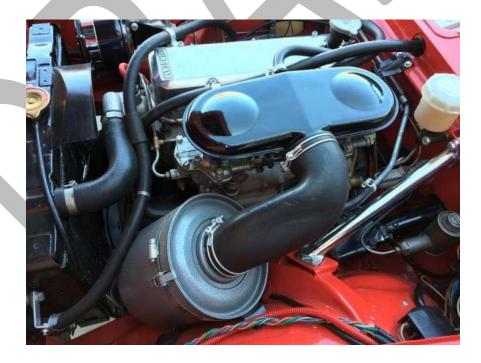
Series 3 and IV GT with Solex Carburetor up to B9410000: Black elbow attaches to large natural aluminum AC canister filter with double wire clamp.
