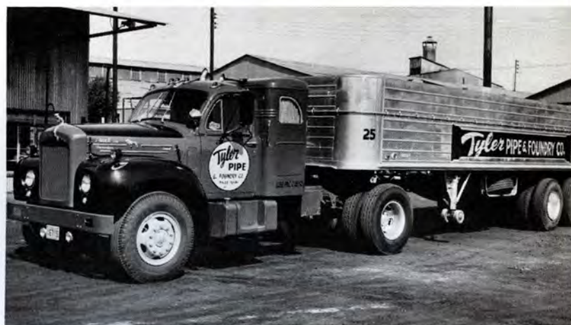
THIS 32-foot grain bed tandem trailer is one of a fleet of 28 Lufkins operated by Tyler Pipe & Foundry
