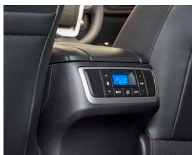
Second row occupants in Limited and Limited ZR grades can chose their preferred air conditioning settings with separate independent controls.
