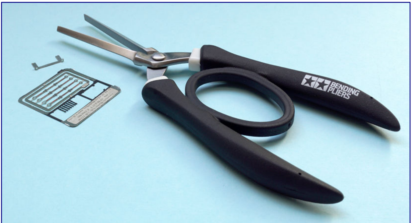
In addition to the Xuron tweezers, the Tamiya bending pliers are particularly useful for the necessary bending work, as shown here with the drilling template.
