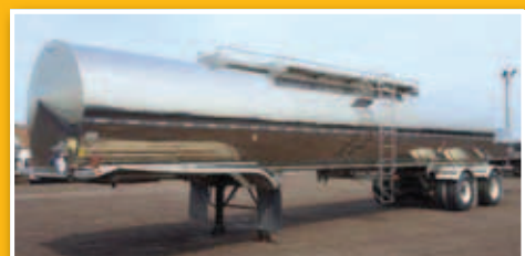
UNIT 10266 - 2009 TREMCAR 26,500 Lts, 2-compt. Stainless sanitary non-code with hyd. 3" pump in rear cabinet.
