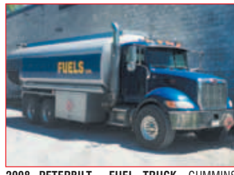
2008 PETERBILT FUEL TRUCK, CUMMINS ENGINE; 300 HORSEPOWER, 10 SPD TRANSMISSION; 20,000 LITRE, BOTTOM LOAD, DUAL PUMPING, MIDCOM COMPUTER. 370,000 KMS. -188897
