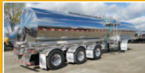
NEW 2017 TREMCAR 8400 USG, DOT-407 stainless one compt. tridem with disc brakes, Michelins, well equipped unit.
