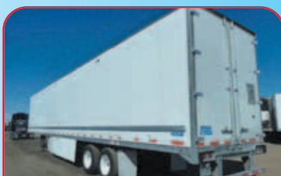
2015 STOUGHTON 53' Z-PLATE PLATE VAN Front And Rear Vents, Sky Lights, Exterior Rub Rail, Air Ride Suspension, 12" Corrugated Steel Scuff Liner, Side Skirts, Like New Condition. -187723
