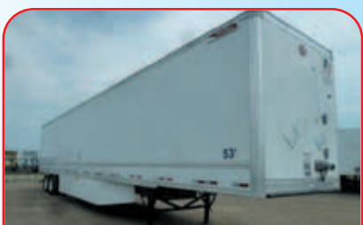
2013 GREAT DANE 53' X 102" PLATE VAN Hendrickson Air Ride Suspension, Front And Rear Vents, Exterior Rub Rail, Side Skirt, Aluminum Roof, Swing Rear Doors, Like New Condition. -273656
