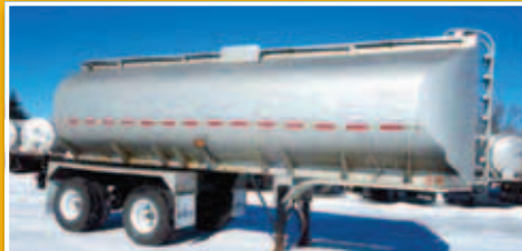
UNIT 10160 - 1990 HUTCH 27,000L, aluminum single compt, non-code pup, 72" spring ride, O.A length 27'. Safetied.
