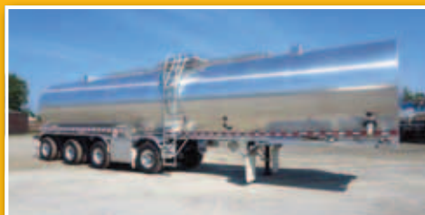
UNIT 10260 - 2017 NEW REMTEC 49,000 Lts, TC-406, convertible aluminum insulated with heat coils, pump-off line, Michelin's. Call
