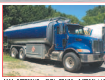
2006 PETERBILT FUEL TRUCK, CATERPILLAR ENGINE; 10 SPD TRANSMISSION; 20,000 LITER, BOTTOM LOAD, DUAL PUMPING, MIDCOM COMPUTER. 445,000 KMS. -188893
