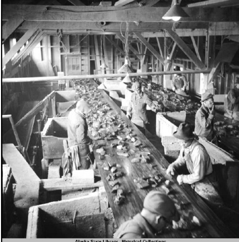
Photo 37. Mine Workers pick white, gold-bearing quartz rock off the sorting belt. AJ mine. Alaska State Library Historical Collections
