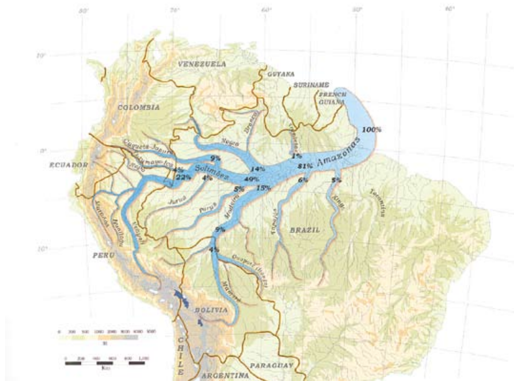
FIGURE 3.2 Percentage contribution of the principal Amazonian hydrographic sub-basins to total basin discharge
