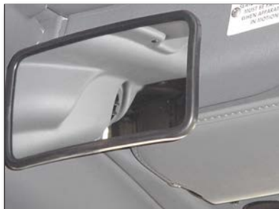
Figure 5.14 – This rearview mirror allows the officer to view occupants in the rear of the cab without having to turn around. (Photo/Mike Wieder)
