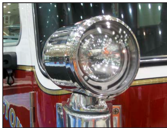
Figure 4.20 – An oscillating warning light. (Photo/Mike Wieder)
