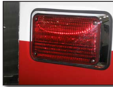
Figure 4.17 – A fixed flasher warning light. (Photo/Mike Wieder)
