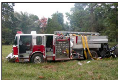
Figure 3.6 – This crash occurred as a result of the right side vehicle wheels leaving the road surface. (Photo/Robert Tutterow, Charlotte, North Carolina, Fire Department)
