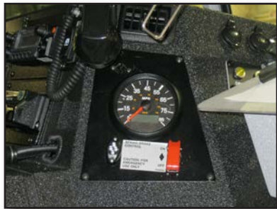
Figure 5.12 – Fire apparatus are equipped with speedometers on the officer's side of the vehicle. (Photo/Mike Wieder)
