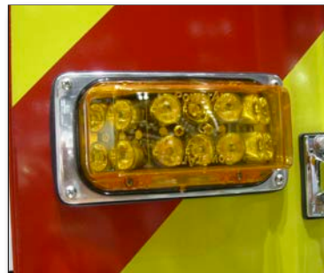
Figure 4.19 – An LED warning light. (Photo/Mike Wieder)
