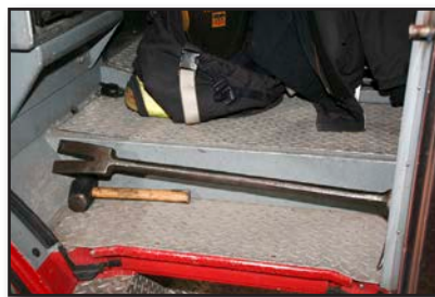
Figure 4.6 – Loose equipment must not be stored inside the apparatus cab. (Photo/ Mike Wieder)
