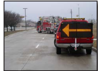
Figures 6.5a and 6.5b – A vehicle-mounted changeable message sign. (Photo/Ron Moore, Plano, Texas)
