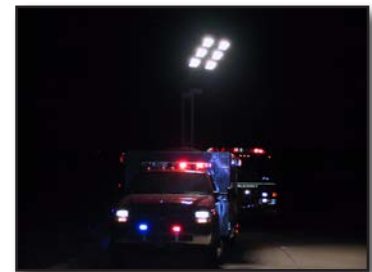
Figure 8.30 – Floodlights should not blind approaching motorists. (Photo/Mike Wieder)
