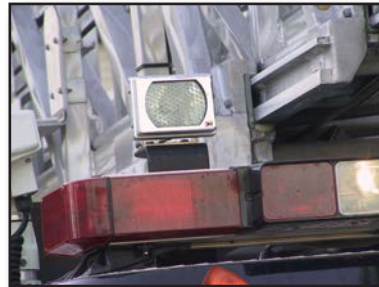
Figure 6.6 – Emergency vehicle may be equipped with emitting devices that trigger a sensor on approaching traffic signals to grant the emergency vehicle the right-of-way. (Photo/Mike Wieder)
