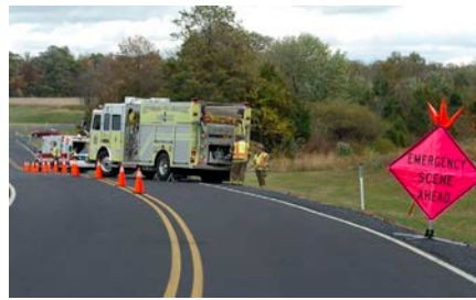
Figure 1.15a — Typical traffic control devices. (Photo/Bob Esposito, Pennsburg, Pennsylvania)
