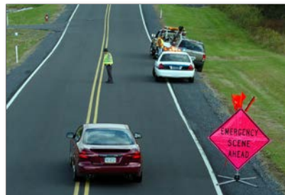
Figure 7.24 – An Emergency Scene Ahead sign. (Photo/Bob Esposito, Pennsburg, Pennsylvania)
