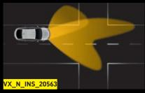
Static cornering light. Spreads light 90 degrees to the left or right to help you see better around corners (up to 25mph, also when reversing).
