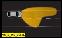
Adverse weather light. Wiper or rain sensor activated for better vision in bad weather conditions (up to 45mph).
