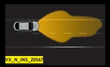
**Motorway light.** 140-metre range, higher and brighter than normal low beam, without dazzle (over 60mph).
