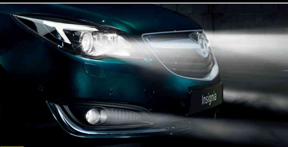
The Insignia can be equipped with the very latest bi-xenon Adaptive Forward Lighting Plus (AFL+) headlight system as an option. This uses a front-mounted camera, rain sensor and steering angle input to improve visibility and safety by automatically adjusting the strength of your headlights to suit different speeds, manoeuvres, weather conditions and traffic situations.
