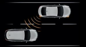
**Side blind spot alert.** This system helps prevent a potential collision with a vehicle in the lane either side of the car by continuously monitoring both blind spots. If a vehicle enters one of those blind spots, a warning light flashes in the relevant door mirror. If you indicate to change lanes, a warning sound alerts you to the potential danger.
