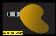
**Town light.** Spreads the beam of light wider and lower. Activated by vehicle speed together with street lighting (20-35mph).
