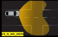
**Pedestrian area light.** Illuminates potential hazards with a wider spread of light – an extra eight degrees left and right (up to 20mph).
