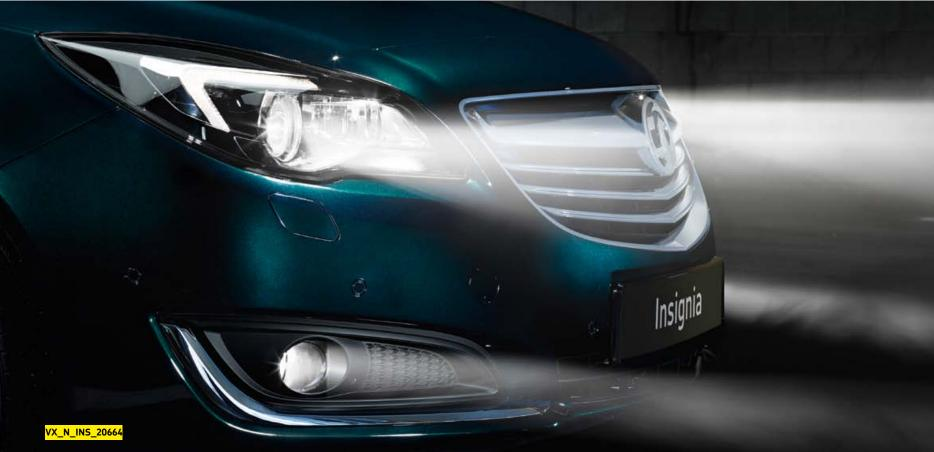
The New Insignia can be equipped with the very latest bi-xenon Adaptive Forward Lighting Plus (AFL+) headlight system as an option. This uses a front-mounted camera, rain sensor and steering angle input to improve visibility and safety by automatically adjusting the strength of your headlights to suit different speeds, manoeuvres, weather conditions and traffic situations.
