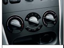
Air conditioning. For chilled air on hot days, faster demisting when it's damp outside, and a more pleasant driving atmosphere throughout the year, air conditioning is a brilliant addition to any car interior. It's standard on Agila SE and optional on S.
