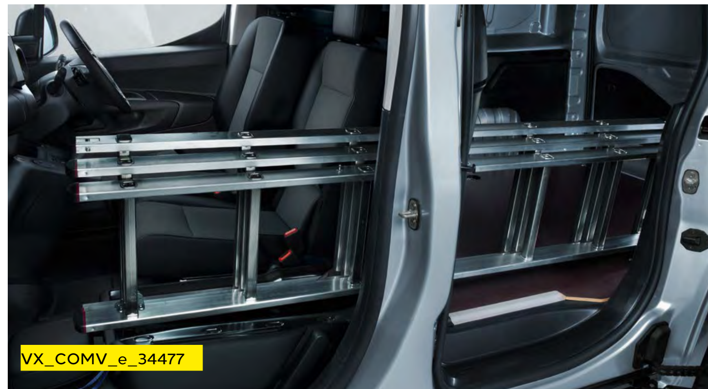
Load-through hatch within bulkhead.
