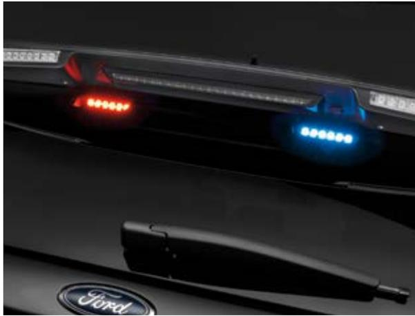
**Rear Lighting Solution (66C).** Includes (2) backlit flashing, linear high-intensity LED lights (driver side red; passenger side blue) with surround cover mounted inside the liftgate glass.
