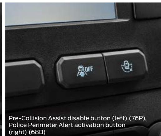
Pre-Collision Assist disable button (left) (76P), Police Perimeter Alert activation button (right) (68B)
