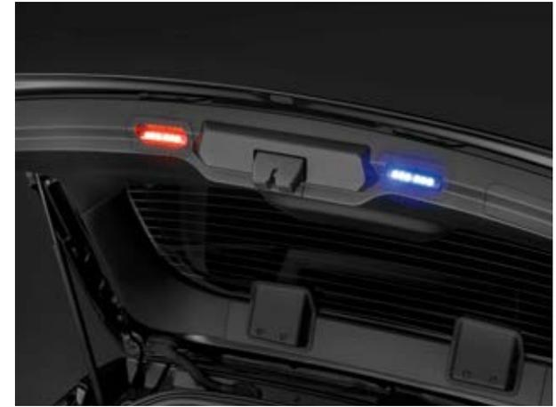
**Police liftgate lights.** Features (2) backlit flashing, linear high-intensity LED lights (driver side red; passenger side blue) mounted inside the liftgate lip; lights activate when liftgate is open.
