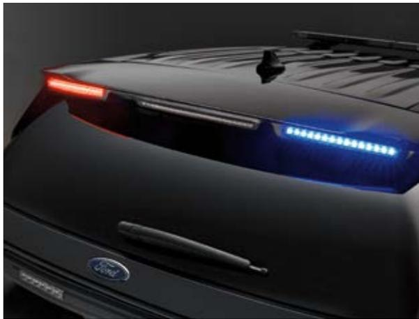
**Rear spoiler LED traffic warning lights (96T).** Includes (2) backlit flashing, linear high-intensity LED lights (driver side red; passenger side blue) mounted on the edge of the rear spoiler. Lights can be programmed for tricolor (red, blue, amber) patterns; also features amber-only traffic direction mode.
