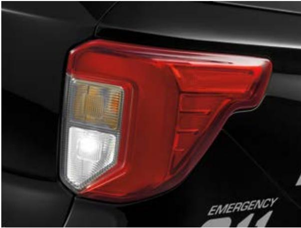
**Taillamp Lighting Solution (66B).** Includes LED base lamps, plus (2) integrated hemispheric lighthouse LED side warning lights.
