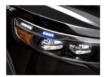
Front Headlamp Lighting Solution (66A). Includes base headlamps with LED high- and low-beam wig-wag function and (2) LED side warning lights (driver side red/white; passenger side blue/white).
