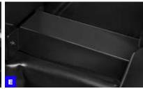
Rear console plate. Interfaces with front console mounting plate and extends through 2nd-row occupant area to seat bottom (acting as wiring conduit on top of transmission tunnel).
