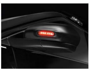
Side marker LED lamps – Sideview mirror (63B). Features backlit flashing, linear high-intensity LED lamps.
