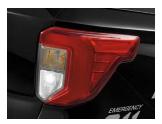
**Taillamp Lighting Solution (66B).** Includes LED base lamps, plus (2) integrated hemispheric lighthead LED side warning lights.
