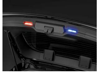
**Rear Lighting Solution (66C).** Includes (2) backlit flashing, linear high-intensity LED lights (driver side red; passenger side blue) with surround cover mounted inside the liftgate glass.
