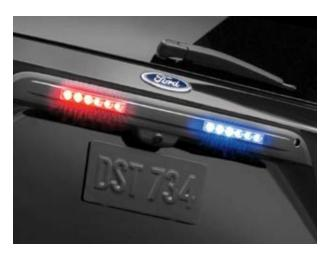
Rear auxiliary liftgate lights (43A). Features backlit flashing, linear high-intensity LED lights (driver side red; passenger side blue) mounted just above the license plate.
