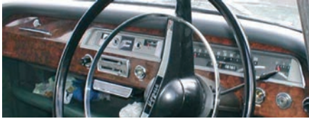
Instrument layout. Note: indicator stalk is on right of steering column; as was usual for most British cars during the 1960s.
