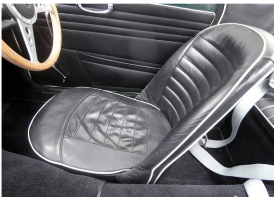
13.7: Early TR4 bucket seats were carried over from the TR3.
