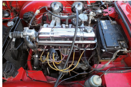
1.2: The nearside of the engine bay. Note the later style oil filler cap.
