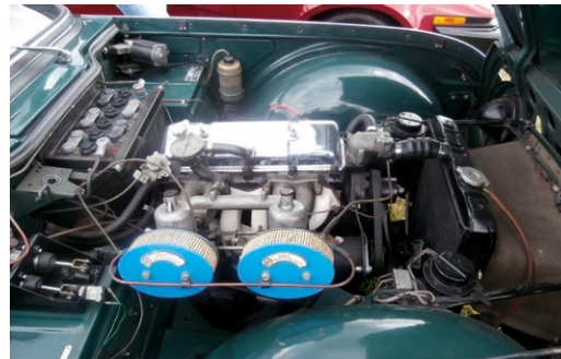
1.3: A view of the engine bay from the offside. Note the twin SU carburetors.
