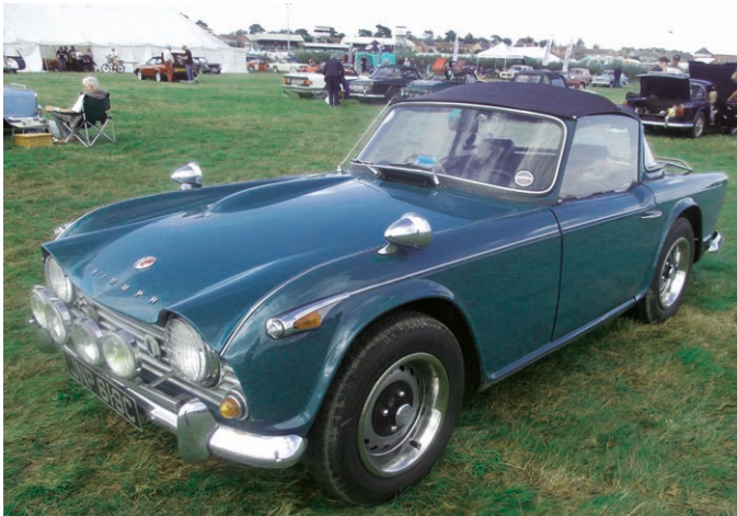
11.1: This TR4A has the wider 5.5in TR6 steel wheels with a 'bling ring' chrome finisher.
