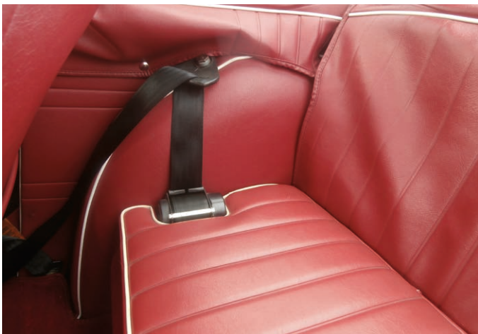
13.8: This is a very neat installation of inertia reel seatbelts on a TR4. The wheelarch mounting is a later fixing point.
