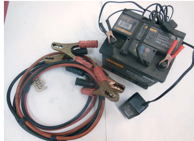
12.3: Use heavy-duty jump leads, and keep a trickle charger nearby if you don't use the car all the time.
