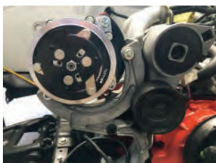
141805 Sanden / R4 multi-groove conversion bracket. (1988-95 Chevy Truck Small Block with Stock Height Valve Covers)
