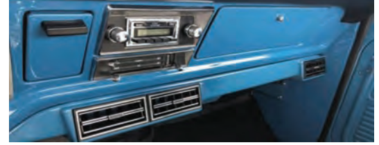
1968-72 factory panel with cable conversion kit and under dash louver package shown
