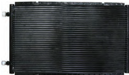
SuperFlow Condensers shown in vertical and horizontal styles. These MUST BE INSTALLED WITH SIDE TANKS IN VERTICAL POSITION ONLY.
