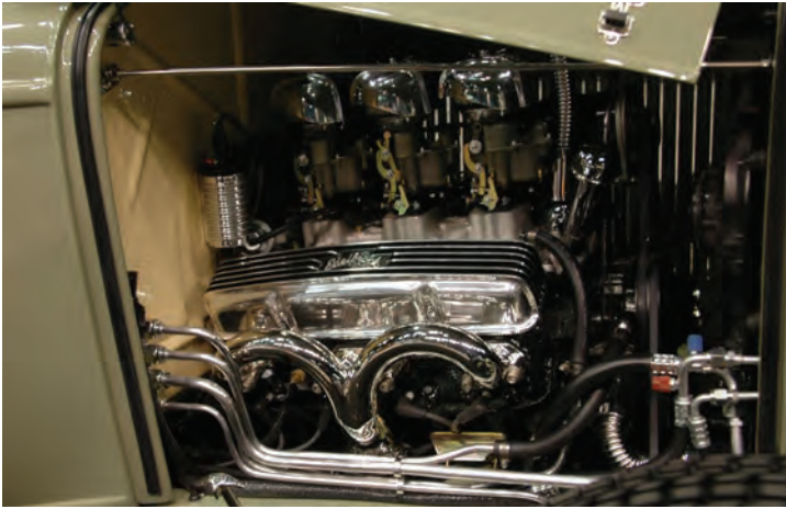
Neatly routed hardlines give your installation a professional look.
