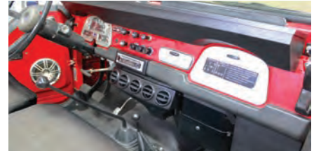
U.S. spec Toyota FJ-40 Land Cruiser dash using factory controls and Vintage Air louvers
