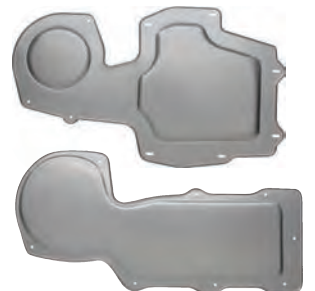
627902 2 - Non-Air stamped firewall blockoff plate. ('67-'69 Camaro, '64-'72 Chevelle & '68-'74 Nova)
