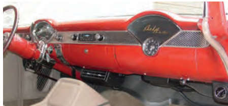
1955-56 Chevy installation with center plenum
