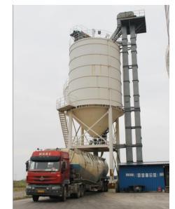
Picture 3. (1)Ash Storage Tank and (2)Surge Bunker
