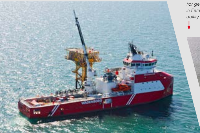
Wagenborg and Royal Niestern Sander developed Kroonborg, a Walk-to-Work Service Operation Vessel (SOV) specialised in the maintenance of offshore systems. The vessel was designed in-house and is the result of the knowledge and experience of the offshore industry and the versatility of Niestern Sander shipyard. The unique vessel design is fully focused on workability, comfort, and safety and was crowned as Vessel of the Year.
