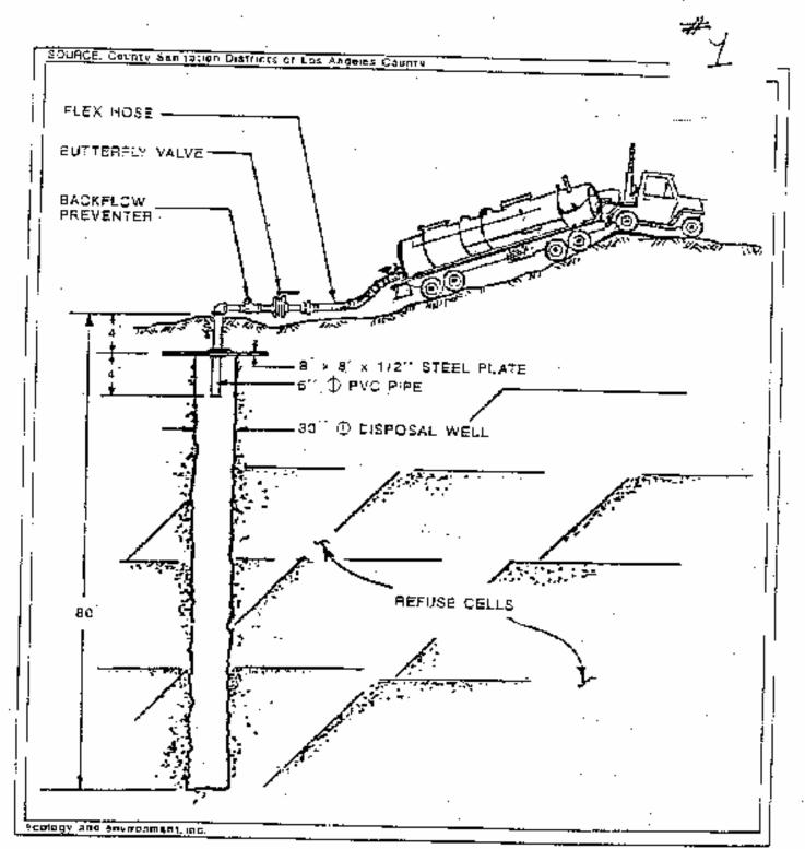
FIGURE 2-4: HAZARDOUS LIQUID WASTE DISPOSAL METHOD Used at the Calabasas Landfill from 1965 to 1980
