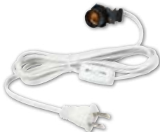
6' Cord Set with Snap-In Pigtail Candelabra Base Socket and Cord Switch *23305 - White 70108 - White No. 18-2, SPT-1, 105° Wire 75 Watts, 125 Volts Snap-In Spring Fits 1" Hole Switch is 12" from Socket
