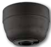
Cathedral Ceiling Canopy Kit 70032 Oil Rubbed Bronze Finish Use With 1/2" or 3/4" I.D. Down Rods Can be mounted onto a cathedral ceiling with up to a 45° angle with or without remote. 85 lb. Load Rating
