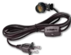
6' Cord Set with Snap-In Pigtail Candelabra Base Socket and Cord Switch *23306 - Brown 70003 - Brown No. 18-2, SPT-1, 105° Wire 75 Watts, 125 Volts Snap-In Spring Fits 1" Hole Switch is 12" from Socket
