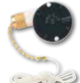
77021 3-Speed Fan Switch Polished Brass Finish Pull Chain Single Capacitor 4-Wire Unit 2' Braided Cord 3A, 250 VAC 6A, 125 VAC
