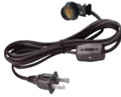
*23306 - Brown 70003 - Brown 6' Cord Set with Snap-In Pigtail Candelabra Base Socket and Cord Switch No. 18-2, SPT-1, 105" Wire 75 Watts, 125 Volts Snap-In Spring Fits 1" Hole Switch is 12" from Socket
