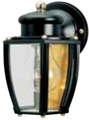
66961 Wall Fixture Matte Black Finish Clear Curved Glass Panels Height: 7.75" Width: 6.00" Extends: 6.50" Height from Center of Outlet Box: 2.25" Back Plate: D: 4.50" Use (1) Medium (E26) Base Lamp, 100 Watt Maximum
