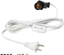
*23305 - White 70108 - White 6' Cord Set with Snap-In Pigtail Candelabra Base Socket and Cord Switch No. 18-2, SPT-1, 105" Wire 75 Watts, 125 Volts Snap-In Spring Fits 1" Hole Switch is 12" from Socket
