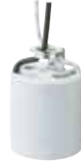
77077 Porcelain Fixture Socket Height: 2.41" 10" Wire Leads Medium Base, 1/8-IP Hickey 18 Gauge, 105° Leads 660 Watts Max., 250 Volts
