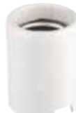
*22282 Porcelain Mogul Base Socket 1500 Watts Max., 600 Volts Height - 2¾" 4 K.V. Pulse Rated
