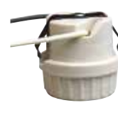
*22212 70424 Porcelain Snap-In Socket Medium Base 6" Wire Leads Fits 1½" Hole 18 Gauge, 125° Leads 660 Watts Max., 250 Volts Height - 1¾"
