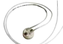
*22472 - GX5.3 Base Mini BiPin Quartz MR16 Socket 12" 18 Gauge Leads SF-1 200° C Leads 100 Watts Max., 250 Volts Height - ¾"
