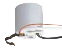
*22372 Porcelain Snap-In Socket Medium Base 9" Wire Leads Fits ¾" x ¾" Hole 18 Gauge, 105° Leads 660 Watts Max., 250 Volts Height - 2"
