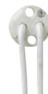
*11104 Porcelain Halogen Socket 5" Wire Leads SF-1 200° C 300V Leads 100 Watts Max., 250 Volts Fits G4, GX5.3, GV5.3 and G6.35 Lamp Bases, Height - ¾"
