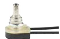
*22306 Push Canopy Switch 4 3/4" Wire Leads 18 Gauge, 105° Leads Fits 3/8" Hole 3A, 250 VAC 6A, 125 VL 6A, 125 VAC Height - 1 1/4"
