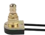
*22303 - Brass Knob Single Pole Rotary Switch with Removable Brass Knob 6" Wire Leads 18 Gauge, 105° Leads 3/16" Nipple, Fits 3/8" Hole 3A, 250 VAC 6A, 125 VL, 6A, 125 VAC Height - 1 1/8"
