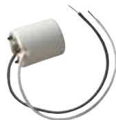
*22480 High Pressure Sodium Lamp Socket 9" Wire Leads Medium Base SF-2/SEW-2 200° Leads 4 K.V. Pulse Rated 660 Watts Max., 600 Volts ½ Screw-Down Height - 1¾"
