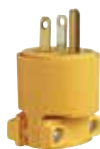
*22633 Heavy Duty Outdoor 3-Prong Plug Plastic Cord Clamp 7/16" Hole 15A, 125 Volts Cord Grip Range 245-700" 12 thm, 18 AWG
