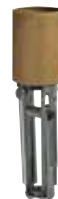
*22138 Adjustable Keyless Socket Medium Base ½-IP Hickey 660 Watts Max., 250 Volts Height Adjustable from 4" - 5¾"
