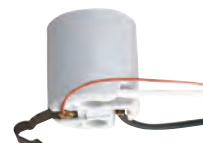
*22372 Porcelain Snap-In Socket Medium Base 9" Wire Leads Fits 3/8" x 1/4" Hole 18 Gauge, 105° Leads 660 Watts Max., 250 Volts Height - 2"
