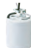
*22370 70425 Porcelain Fixture Socket Medium Base 10" Wire Leads, Height - 2.41" 1/8-IP Hickey 18 Gauge, 105° Leads 660 Watts Max., 250 Volts
