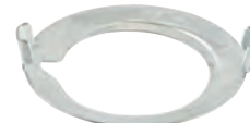
70428 Steel Shade Ring for Medium Base Sockets Ring Size - 2 3/8" Outside Diameter - 2 1/4" Inside Diameter - 1 1/2"
