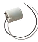
*22480 High Pressure Sodium Lamp Socket 9" Wire Leads Medium Base SF-2/SEW-2 200° Leads 4 K.V. Pulse Rated 660 Watts Max., 600 Volts 1/2" Screw-Down Height - 1 3/4"
