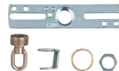
70350 - Brass Finish 70352 - Antique Brass Finish Screw Collar Loop Kit Fits Canopies with a 1 1/8" Center Hole Tapped 1/4"-IP, 35 lb. Load Rating Includes: • 1 Crossbar 4" Long • 1 Screw Collar Loop • 2 Locknuts • 1 Lock Washer • 1/4"-IP x 1 1/2" Nipple • 1 3/8"-IP x 1/4"-IP Reducing Hickey • 2 8-32 x 1/2" Mounting Screws
