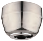
70031 Cathedral Ceiling Fan Canopy Kit Brushed Nickel Finish Use With 1/2" or 3/4" I.D. Down Rods Can be mounted onto a cathedral ceiling with up to a 45° angle with or without remote. 85 lb. Load Rating
