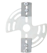
70111 Adjustable All-Purpose Crossbar Slips 3/8"-IP Holes Tapped 8-32 Adjusts from 3 1/8" to 5" for Slot Mounting on 3", 3 1/4" or 4" Box Two 1/2" Head Screws Included Two 1/4" Head Screws Included 35 lb. Load Rating
