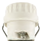
*22276 Porcelain Snap-In Socket Medium Base 660 Watts Max. 250 Volts Height - 1 3/4"
