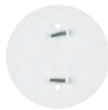
*29452 70065 White Outlet Concealer Holes Spaced 3 ½" Apart Diameter - 4¾" Holes Spaced 3 ½" Apart Mounts on 4" Outlet Box Includes: • 2 8-32 x ¾" White Head Screws *Polybagged Bulk Items
