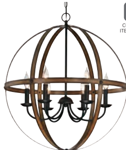
63336 Stella Mira 6 Light Chandelier Barnwood and Oil Rubbed Bronze Finish Height: 27.00" Diameter: 24.00" Chain: 36" Cord: 60" Use (6) Candelabra (E12) Base Lamps, 40 Watt Maximum
