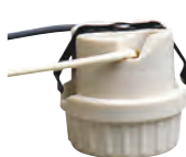
*22212 70424 Porcelain Snap-In Socket Medium Base 6" Wire Leads Fits 1 1/2" Hole 18 Gauge, 125° Leads 660 Watts Max., 250 Volts Height - 1 3/4"
