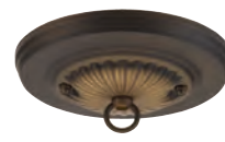
70050 Traditional Canopy Kit with Center Hole Oil Rubbed Bronze Finish 5½" Diameter, 7/16" Center Hole 50 lb. Load Rating Includes: 1 Canopy • 1 Crossbar • 4 Mounting Screws • 1 Lock Washer • 1 Locknut • 1 Screw Collar Loop • 2 Cap Nuts
