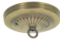
70053 Traditional Canopy Kit with Center Hole Antique Brass Finish 5½" Diameter, 7/16" Center Hole 50 lb. Load Rating Includes: 1 Canopy • 1 Crossbar • 4 Mounting Screws • 1 Lock Washer • 1 Locknut, 1 Screw Collar Loop • 2 Cap Nuts
