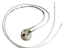
*22470 - GY6.35 Base Mini BiPin Quartz MR16 Socket 12" 18 Gauge Leads SF-1 200° C Leads 100 Watts Max., 250 Volts Height - 3/8"
