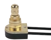
* 22303 - Brass Knob Single Pole Rotary Switch with Removable Brass Knob 6" Wire Leads 18 Gauge, 105° Leads 7/16" Nipple, Fits 3/8" Hole 3A, 250 VAC 6A, 125 VL, 6A, 125 VAC Height - 1 1/4"
