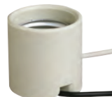
*22218 Porcelain Keyless Socket 1 Screw Surface Mount Medium Base 7" Wire Leads 660 Watts Max., 250 Volts 105° Leads, Leads Height - 1 5/8"
