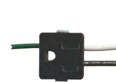
*22532 Snap-in Outlet with Ground Wire Black 6" Wire Leads 14 Gauge 15A, 125 Volts Fits 1" Square Opening with Green Ground Wire Height - 3/8"
