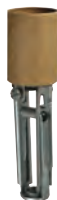
*22138 Adjustable Keyless Socket Medium Base 1/8-IP Hickey 660 Watts Max., 250 Volts Height Adjustable from 4" - 5 5/8"
