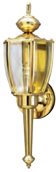
66924 Wall Fixture Polished Brass Finish Clear Curved Beveled Glass Panels Height: 18.50" Width: 5.75" Extends: 6.00" Height from Center of Outlet Box: 11.50" Back Plate: D: 4.50" Use (1) Medium (E26) Base Lamp, 100 Watt Maximum
