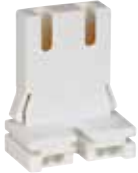
*22457 Medium BiPin Lamp Holder Floating Action for U-Shape Lamps Low Profile Size 20 Gauge 660 Watts Max., 600 Volts Non Shunted
