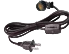
70003 - Brown 6' Cord Set with Snap-In Pigtail Candelabra Base Socket and Cord Switch No. 18-2, SPT-1, 105" Wire 75 Watts, 125 Volts Snap-In Spring Fits 1" Hole Switch is 12" from Socket
