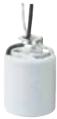
77077 Porcelain Fixture Socket Height: 2.41" 10" Wire Leads Medium Base, 1/8-IP Hickey 18 Gauge, 105° Leads 660 Watts Max., 250 Volts
