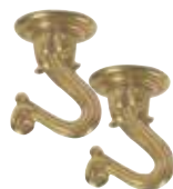
70450 1 1/2" Swag Hook Kit Polished Brass Finish Includes: • 2 Hooks • 2 Spring Toggle Wings • 2 Running Thread Studs: #10-24 x 2 7/8" • 2 Wood Screws: #10 x 1 1/4" • 30 lb. Load Rating
