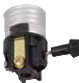
*22504 3-Way Turn-Knob Socket Medium Base 250 Watts Max. 250 Volts Height - 1½"
