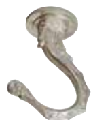
70446 Large 2 1/2" Swag Hook Kit Brushed Pewter Finish Includes: • 1 Hook • 1 Spring Toggle Wing • 1 Running Thread Stud: 1/4-20 x 2 7/8" • 1 Wood Screw: #14 x 1 3/8" • 45 lb. Load Rating
