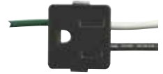
*22532 Snap-in Outlet with Ground Wire Black 6" Wire Leads 14 Gauge 15A, 125 Volts Fits 1" Square Opening with Green Ground Wire Height - 7/8"
