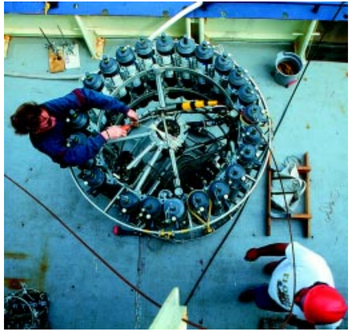
Laura Stein rigs a conductivity/temperature/depth rosette sampler in preparation for an Oceanus cruise in summer 1996.
