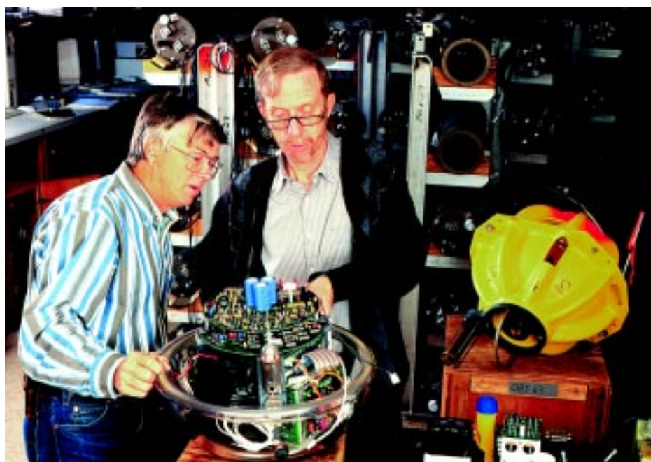
Beecher Wooding, left, and Ken Peal set up an ocean bottom seismic recorder. Another recorder, fully rigged for deployment with yellow “hardhat” and spotting flag, is at right.
