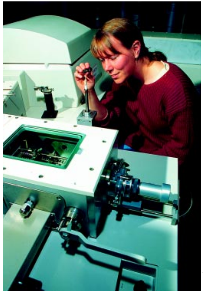
Joint Program student Elizabeth Minor repairs the sample probe on the mass spectrometer she uses to obtain molecular-level information on lipids, sugars, proteins, and other natural and synthetic substances in oceanic organic matter.
