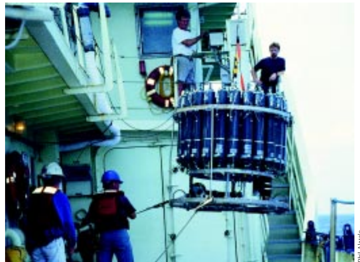
Scientists and crew swing a conductivity/temperature/depth rosette sampler into action during Oceanus Voyage 279 in summer 1996.
