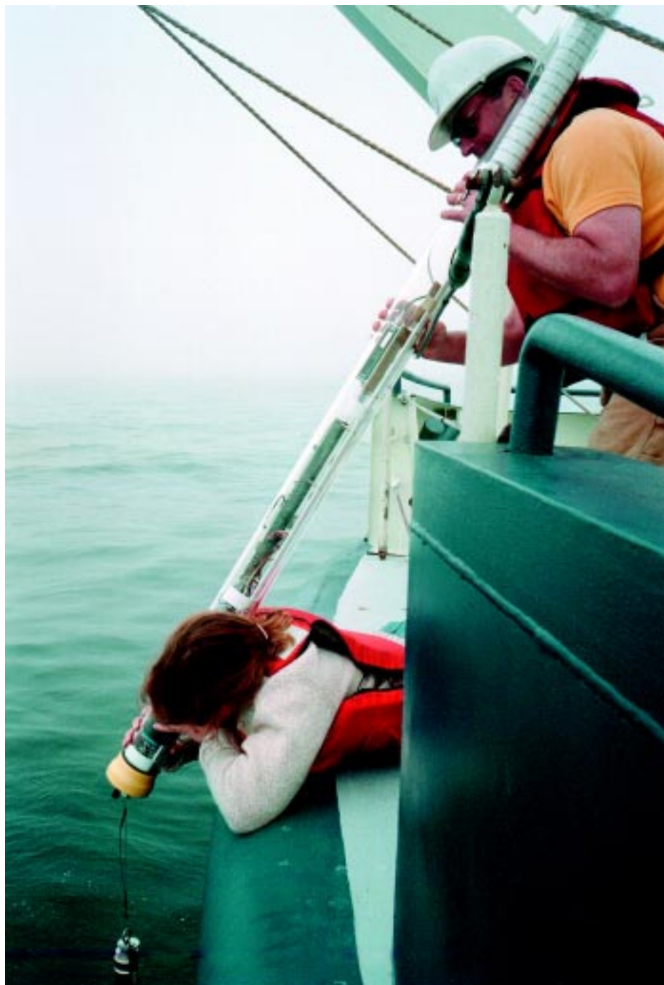
Amy Bower and Fred Grosse of Susquehanna University launch a RAFOS float from R/V Oceanus.
