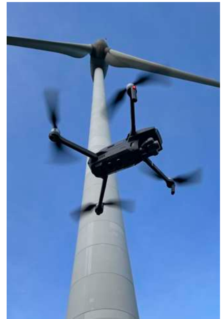
The SkyVisor drone taking off to start the automatic inspection
