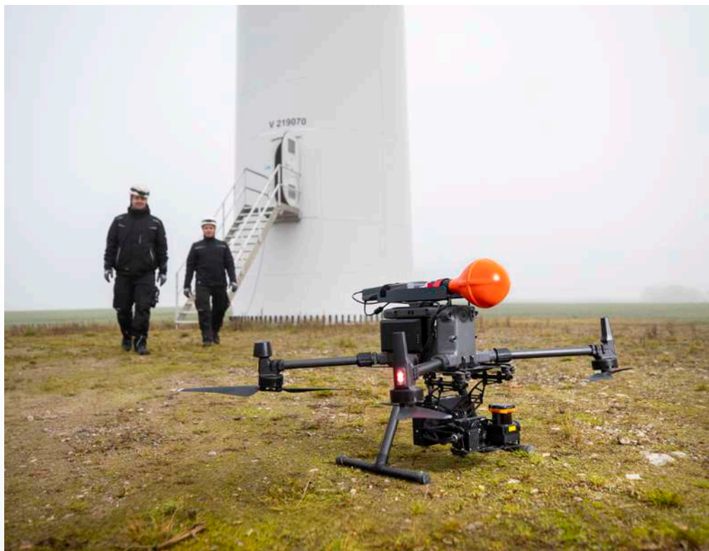
Picture of a ready-to-use drone for rotor blade inspection and contactless lightning protection system inspection
