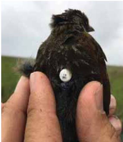
A seaside sparrow fitted with a miniature VHF transmitter for tracking purposes.
