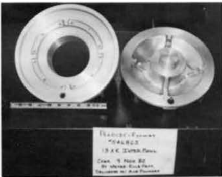
Alum core box for high production pump bowl
