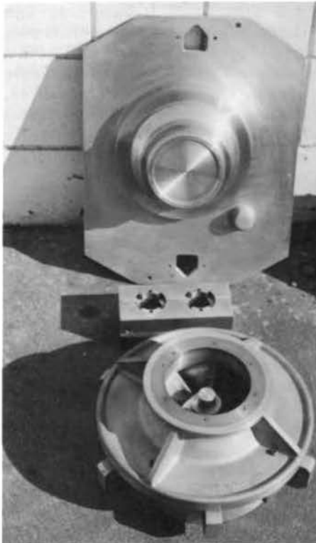
High production alum and brass pattern for pump impeller.
