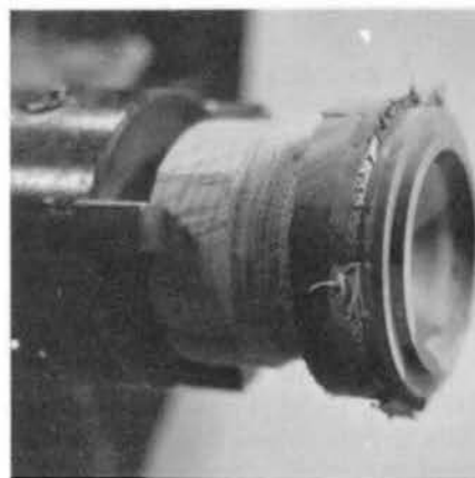
Lip turned in bottom section to fit cylinder section. Ready to part off and reverse chuck
