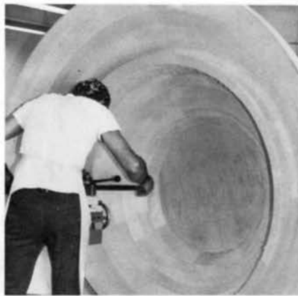
Gene Meyer turning a tool holder for a large milling machine.
