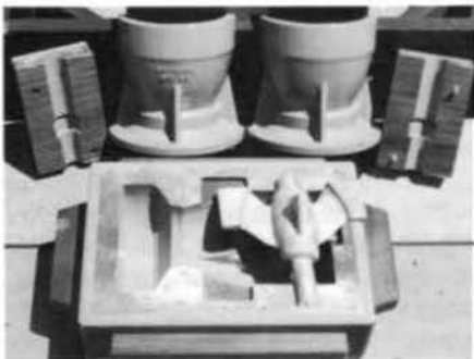
Mahogany pattern equipment for pump section case.
