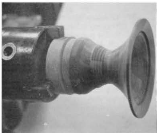
Birdhouse roof partly turned. Note ample material to prevent chatter
