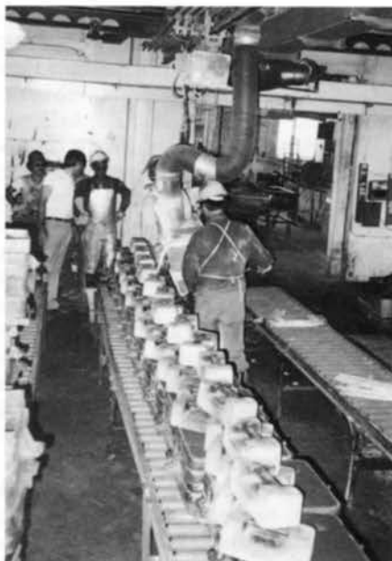
Foundry pouring brass for vanes to be used in production impeller pattern.
