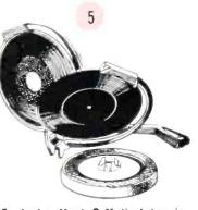
Exclusive Mech-O-Matic Intermix Completely automatic changer intermixes 7" LP albums, 33½, 45 RPM stereo-monaural records in any bank, any sequence. No wires, microswitches, electronic aids for changing motor speeds or spindle sizes.
