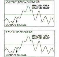
of our commitment to design excellence. Its three-stage signal path optimizes the sonic advantages of traditional push-pull amplifier circuits. By combining a multiple level DC power supply with conventional power transformers and rectifiers, we've improved on previous efforts at increasing heat efficiency—anticipating the benefits of "Class D" and "smart power supply amplifiers, without relying on unproven technology. This has enabled us to build a power amp that is more
