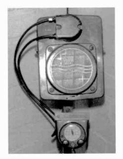
PHILIPS AUTO RADIO – This is one of the earliest automobile radios manufactured by Philips Lamps, Ltd., of Surrey, England. This unique display on a vertical post shows the receiver and speaker unit mounted on a stand with cables connected to the tuning head below. The tuner unit was mounted on the steering wheel post or the dashboard to enable the operator to tune the radio while driving the automobile. (Girard Faassen – Reuver, Holland)
