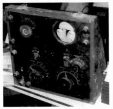
A DeForest BC-98, (ca. 1920). This 3-tube, World War I receiver used VT-type tubes and paired up to a matching transmitter. Just try to find the automotive clock that went in the upper right hole. It sold without tubes, clock, or the back half cover lid for \$1301
