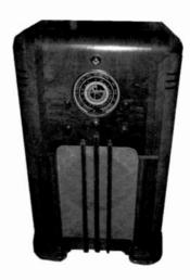
Figure 3. Sparton produced a number of console models. This Model 867 is an 8-tube console with a rated audio output of 7 watts. It tuned the broadcast and SW bands.
