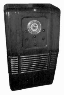
Figure 9. Sparton of Canada offered a 15-tube set also housed in an unusual cabinet. It covered the BC, SW and weather bands.
