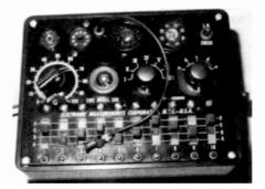
Figure 1. The top panel of the EMC 208 tube tester. The grid cap clip is probably not original.
