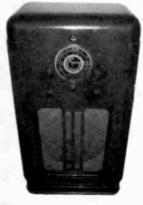
Figure 5. The Model 1167, an 11-tube set, is similar in appearance to the Model 867. In addition to the broadcast and SW bands, the radio also tunes the 140-420 kHz weather band.
