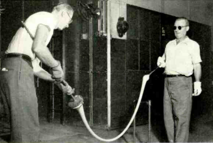
A ball of molten glass is drawn between rods down a 100 ft. corridor until it is no bigger around than your finger.
