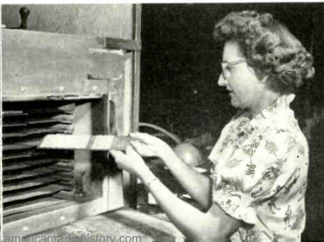
Newly painted lamp caps go into an oven for pre-heating. In an even hotter oven characters are baked until they attain a hard, glossy finish.
