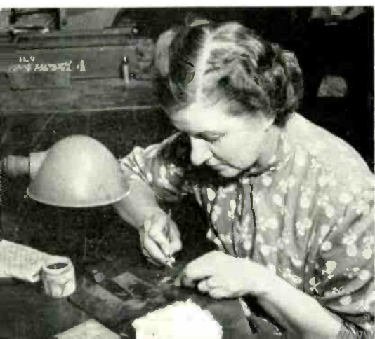
Standard characters are embossed on caps mechanically, filled with glaze and baked. Special symbols must be hand painted.
