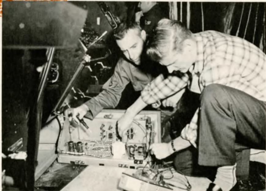
TechRep and airman work together in trouble shooting a component of the FPS-6B radar at the 777th AC&W Squadron, Klamath, California.
