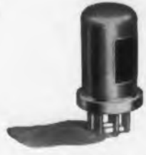
The Edison Control Relay Amplifies Power 500,000 Times
