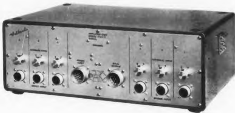
Fig. 3. The back of the amplifier case. The bridge circuit is etched into the panel. Connectors for all cables have been selected so that it is impossible to connect them to the wrong terminal.
