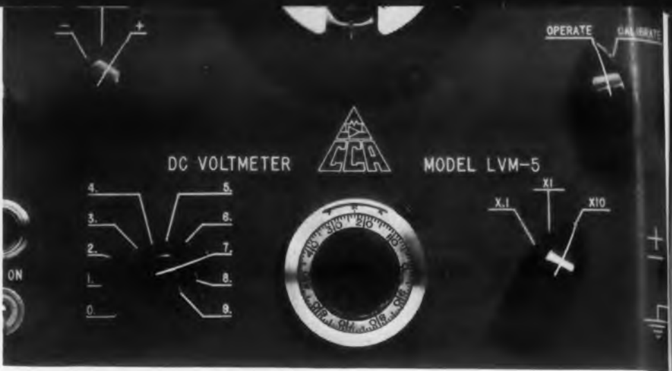
Fig. 1. Closeup of the face of the voltmeter showing an unknown voltage of 7.624 \times 10 = 76.23\text{v} read from the attenuator.
