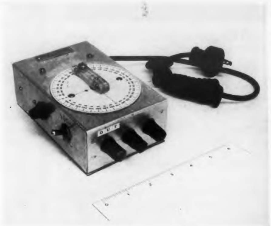
Fig. 1. One version of the laboratory phase comparator.
