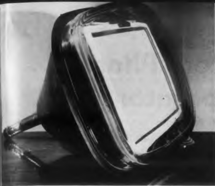
Fig. 1. The rectangular-picture "Chromatron" which employs a single-gun construction.
