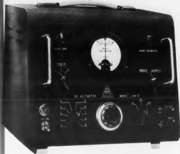
Fig. 3. Portable version of the Model LVM-5 laboratory voltmeter.
