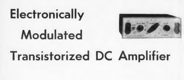
MODULATED entirely by electronic means, this all-transistor de amplifier has no mechanical chopper to introduce problems of noise, maintenance and wear. The eleven transistor unit provides sufficient gain to drive most galvanometric recorders from millivolt signals. Since no vacuum tubes are used, the unit is reliable, requires no warm-up time, and quickly stabilizes itself. A floating input allows the amplifier to operate from any source resistance.
