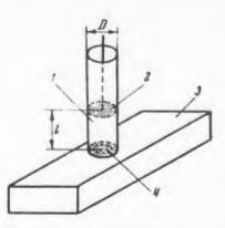
Fig. 2. Subcritical cavity arrangement: 1. Subcritical waveguide; 2. Piston; 3. Main lines 4. Capacitive diaphragm (window).
