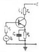
**Fig. 1.** A sharp drop in the input pulse increases the influx of carriers at the output of the circuit, thereby decreasing the buildup time of the wavefront.
