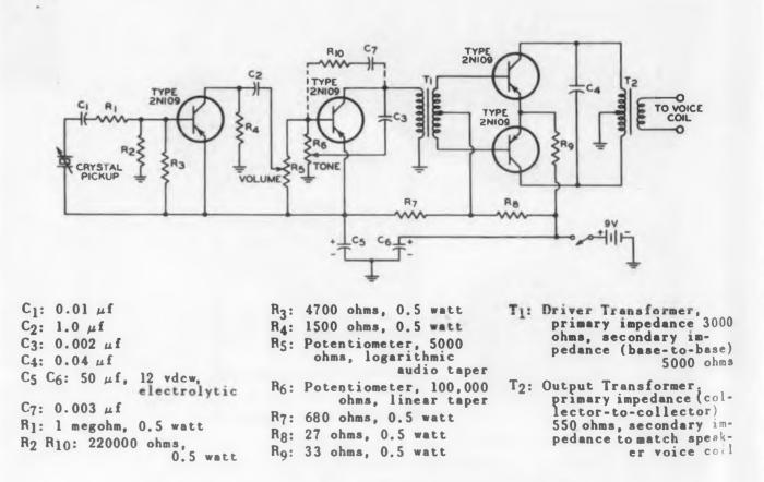
Fig. 1. Circuit of the transistor battery-powered phonograph amplifier.
