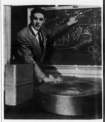
Electron Storage Vault: A low inductance capacitor for energy storage, built by General Electric Co., is shown at right. The unit is rated at 100 kv, 0.25  $\mu$ f, and has a ringing frequency of 2.5 mc. The existing standard type of energy storage capacitor, shown at left, is rated 20 kv, 7.5  $\mu$ f, and has a ringing frequency of 200 Kc.
