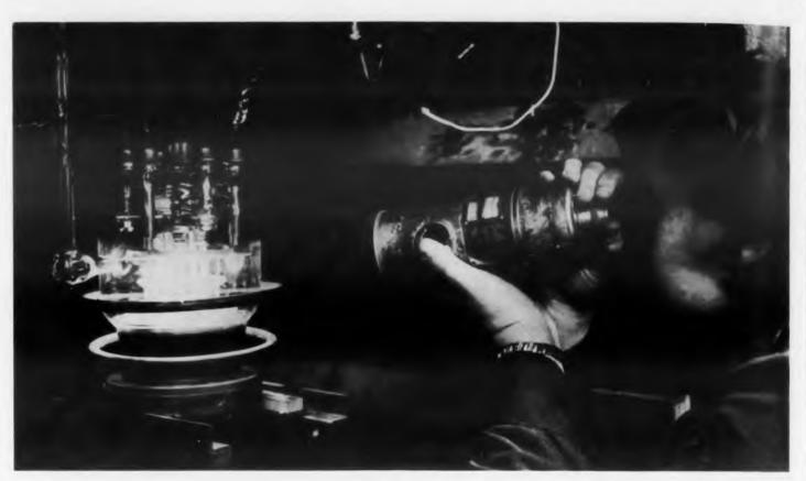
Specialized industrial tubes manufactured in small numbers are evacuated in special ovens. Operator is checking temperature of tube (WL-5936 triode) as it is evacuated.
