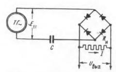
5. The bridge and capacitor convert the tach-generator output into a dc signal portional to the tach-generator speed.
