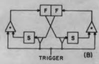
Fig. 1. Logical diagrams of unconditional steering (A), and conditional steering (B). In A the reversal of the steering gates after the change of flip-flop state is unconditional, while in B it is conditional upon removal of the trigger.
