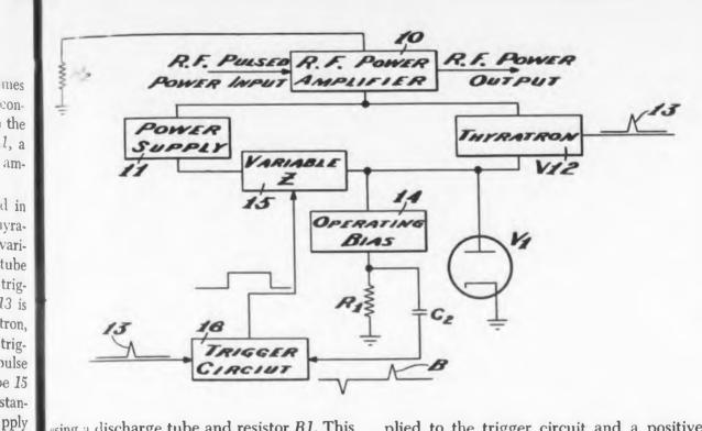
using a discharge tube and resistor R1. This impedance controls the operating point of the amplifier during conduction. By controling the bias on its grid the shape of the output wave may be altered.
