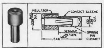
PRINTED CIRCUIT TEST JACKS
