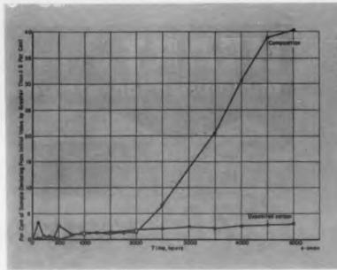
Fig. 4 Load-Life Characteristics For Most Stable Group of Composition and Deposited-Carbon Resistors
