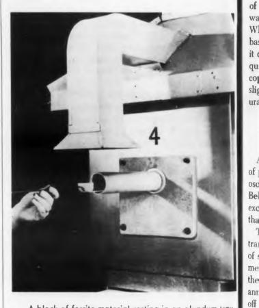
A block of ferrite material resting in an alundum tray is being inserted in a furnace for firing. The material has been improved by adding copper and manganese in proper quantities to the basic ferrite. Copper increases the reactivity of the mixture and thus decreases the firing temperature by at least 100 C. The manganese addition lowers the conductivity, making possible smaller dielectric loss.
