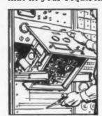
Five seconds to put chassis in testing position. Slides smoothly out of rack, locks. Pivoting mechanism brings underchassis parts to easiest working angle. Functioning of unit need not be interrupted!
