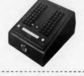
LIBRASCOPE PUNCHED CARD CON-VERTER — This relay-operated converter accepts three-decimal digit and sign, two channel, IBM punched card information and converts it to analog form for input to XY plotters. Cards can be manually fed through the IBM reading brushes one at a time or automatically read at rates to 50 cards per minute with an accuracy of 0.1%.
