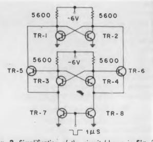
Fig. 3. Simplification of the circuit (shown in Fig. 2. Dc storage has been removed and the bottom transistors of the two-element series gates are time shared.
