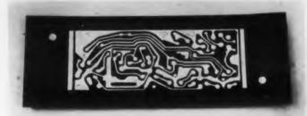
Two steps in making printed circuits are shown. Copper is first punched into the molding board and then excess copper is stripped away. Later the board is cured in a compression mold.
