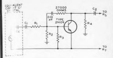
Fig. 6. Alternative input circuit for use with pickups having flat frequency-response characteristics.
