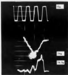
Figure 2. Oscillogram for shock test along vertical axis for an integral mounting system carrying two, six-pound electronic units. Upper trace: amplitude calibration at 60 cps. Middle trace: output from mockup of equipment. Lower trace: input to mounting assembly.
