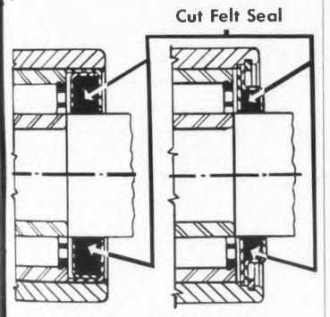
Suggested Application of Felt for Use in Metal Stamping Seals for Pre-Lubricating Ball Bearings
