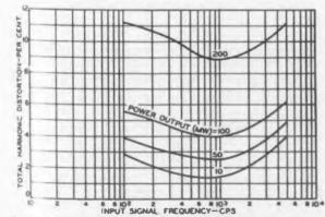
3. Total harmonic distortion produced by implifier at various output power levels.
