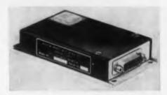
The REL-102 instrumentation amplifier covers the subsonic, sonic and ultrasonic regions. The design accomplishes the function of amplifying and impedance transforming low level signals from transducers, to a level and an impedance suitable to drive a transmission line, subcarrier oscillator, direct writing recorder or an oscillograph recorder at a considerable distance from the pick-up.
