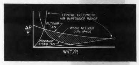
Altivar induction motor fans increase speed 3 to 5 times from sea level to 70,000 ft. Send for Catalog Sheet 30101-3
