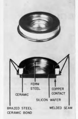
ACTUAL SIZE view shows G-E silicon rectifier cell hermetically sealed to better protect the silicon
