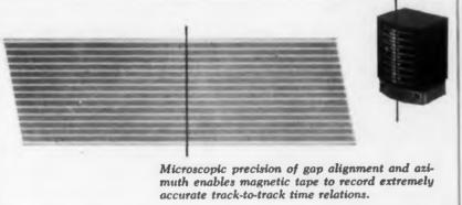
For time correlation the head stacks on an Ampex Tape Recorder are like an "electronic tee-square." All of the gaps are in line within 1/10,000th inch. And gap azimuth is accurate to a minute of arc. Tape moves past the head at speeds up to 60 inches per second and multiplies the track-to-track timing accuracy accordingly. (But consult us at Ampex before you rely on simple arithmetical conclusions).
