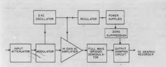
Fig. 3. Block diagram of the dc amplifier. The transistor regulator lengthens battery life to 200 hours or regulates wide fluctuation in ac line voltage.
