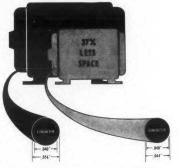
Two imaginary motors are shown, one using conventional Teflon coated magnet wire (left), and the other using the same size wire with Fused Film insulation, (right). The size of the motor would actually be further reduced since Fused Film makes supplementary insulation unnecessary.
