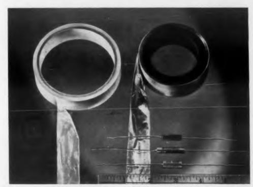
with and without a vacuum-deposited layer of aluminum. (Capacitors by Balco Research Laboratories, Inc., Newark, N. J.; films by Dilectrix Corporation, Farmingdale, L. I., N. Y.) Many electronic components can be redesigned to take advantage of the unique properties of Teflon tetra-fluoroethylene resins. Major directions are toward higher temperature limits and miniaturization.
