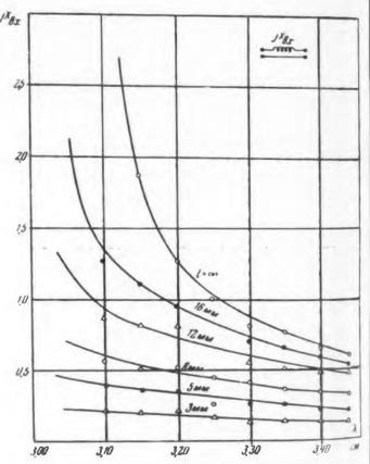
Fig. 3. Experimentally measured input impedance of round subcritical 18mm waveguide. The ordinate, jX<sub>1n</sub>, is the impedance relative to that without the piston. At upper right is the simplified equivalent diagram.
