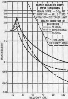
gure 1. Graph showing specified limits of isolation efficiency during missile launching and the performance of distributed-element mounting system.
