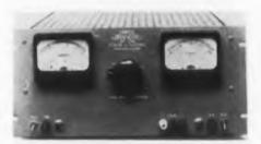
This magnetic amplifier controlled dc power supply, Model C169, has a voltage range of 0 to 150 v, at currents from 0 to 1-1/2 amp. The unit is regulated to ±1 per cent for line or load, with a compensating adjustment control to secure positive or negative impedance, thus giving 0 per cent load regulation. Ripple is 0.1 per cent for all line or load conditions. Transient response is better than 0.2 see. Line input range is from 105 to 125 v ac at
