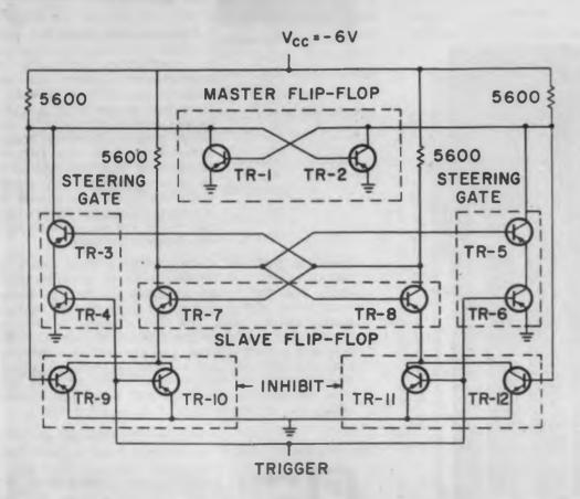
Fig. 2. Circuit illustrating the concept of conditional steering. Its operation is based on a second or "slave" internal flip-flop serving as the memory element.
