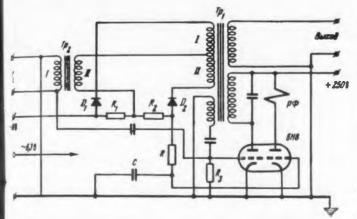
Fig. 4. Narrow-band frequency relay (filter) combined with oscillator. In the absence of a signal  $(f_c)$  the double diode is blocked by the 16v bias.
