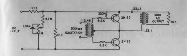
Fig. 1. Complete schematic of the transistor modulator. Since the input signal is in effect the supply voltage for the modulator, the complete output characteristics are shown in Fig. 2.
