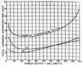
Fig. 4. Total harmonic distortion produced by the amplifier as function of power output.
