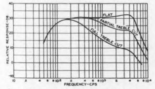
Fig. 2. Response of amplifier and crystal pickup.
