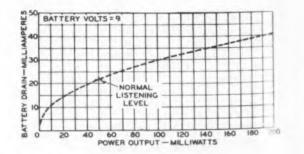
**Fig. 5.** Total current drawn by the amplifier as a function of power output.
